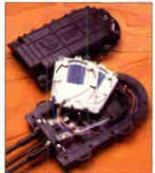
The Runt measures 8.5 x 14.75 inches and can be used in aerial, buried and underground applications. Its fiber management system is molded into the bottom shell half, providing separate areas for routing and protecting buffer tubes from loose cables or bare fibers from unitube type cables and allows for the splicing of loose-tube and unitube cables in the same closure.
