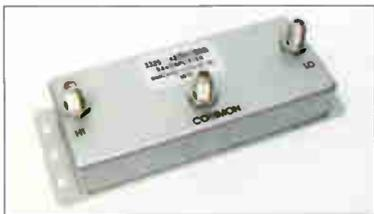
MHz). Model 3329-42/54, typical of this series, splits the low passband at 5-42 MHz and the high passband at 54-1000 MHz, with typical insertion loss of 1.0 dB (3.0 dB at 42 and 54 MHz). Mutual isolation is 30 dB, with standard 75 ohm, type "F" connectors.
