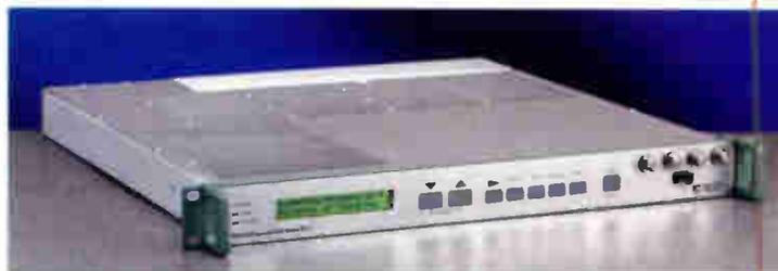
S-A’s UC-4 Universal Upconverter contains Broadband Innovations’ efficient upconverter modules.
