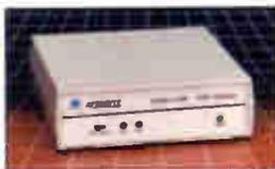
Model 3340 has reliable operation up to 100 meters and does so by encoding the RS-232 data before transmitting on the POF cable. The signal is decoded and restored at the receiver to the original transmission. The device comes with a 10-foot DB9 extension cable.
