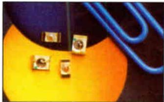
Lumex Inc.'s surface mount technology (SMT) light emitting diodes (LEDs) feature a built-in domed lens on top of a flat-bottomed carrier. Lumex LEDs focus the light to a 50-degree angle of emission, vs. a conventional angle of 130 to 180 degrees. These LEDs are designed for display or backlighting applications, as well as status or circuit fault indicators.
