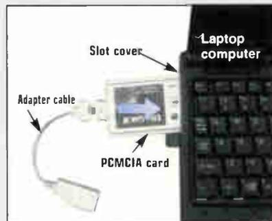
Figure 5: Inserting PCMCIA card into slot
