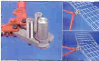
The attachment can create a multitude of Flextray fittings. It works by placing the Cleanshear cutter with attachments between prepared sections of Flextray. By pushing the handles together, the tray bends evenly to the desired radius. The Flextray's wire mesh cable management system provides on-site flexibility and aids in faster installation.
