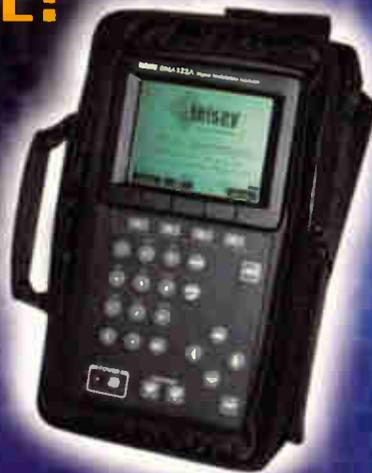
With 16, 64, 256 QAM and a 5-860 MHz input band, the Telsey DMA 122 Enhanced has an RF analog range up to 60dBmV, a fast all channel sweep and the capability for IF measurements. Other features include enhanced sensitivity, a selectable internal low noise input amplifier, and easy menu driven navigation, all housed in a very rugged handheld device with a rechargeable NiMh battery.
