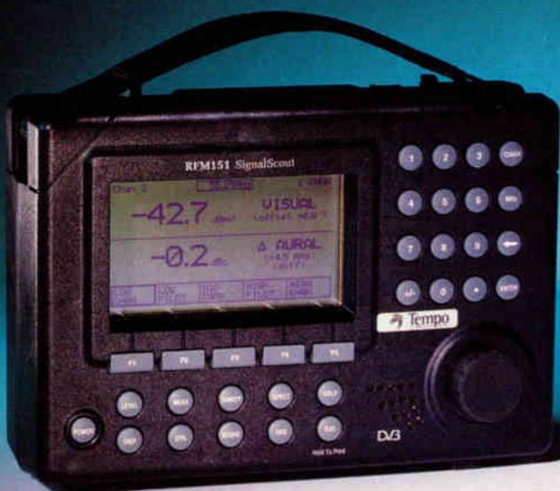
When it comes to troubleshooting and locating return path ingress, Tempo's RFM151 Broadband Analyzer gives reason to celebrate. With its unique Ingress Monitor Mode and ability to minimize forward path signal overload, low level ingress measurements can be made in common path locations — resulting in superb ingress detection. Try Tempo's RFM151 today and you'll be enjoying many happy returns.
