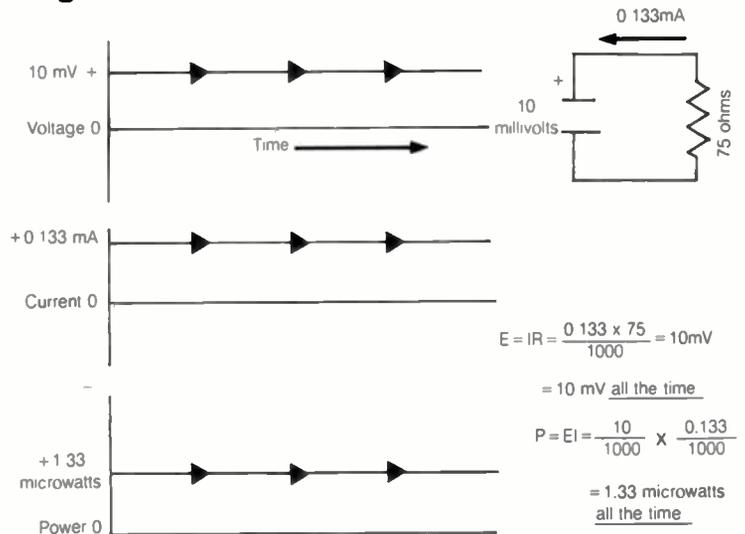
In a dc circuit like this everything is easy, because all the quantities are constant. The voltage is 10 millivolts (all the time), the current is 0.133 mA (all the time) and the power is constant. There is no difficulty agreeing on what each quantity means in this situation.
