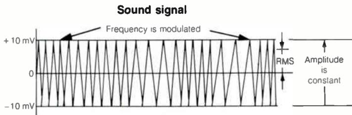
of the RMS voltage present, just like a c-w signal, its effective voltage being 0.707 x the peak voltage.
