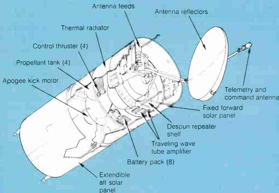
prove the commercial viability of worldwide satellite communications. The Intelsat 1 had an 18-month design life and Intelsat 2 was a three-year bird. Both were operational well beyond their design life and were removed from service because of the availability of superior performance from Intelsat 3 and Intelsat 4 satellites.
