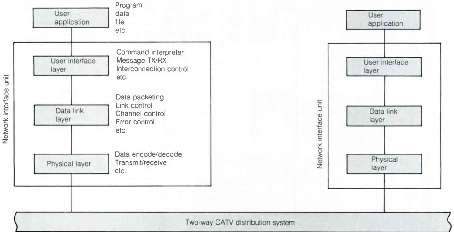
cast" downstream data, identifying data packets addressed to it, transferring the associated data to the user device. A block diagram of the NIU is shown in Figure 4.
