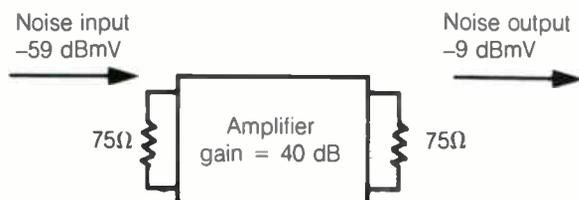
If the amplifier had no internal noise, the noise output would be the input noise (dBmV) plus the amplifier gain (dB).
