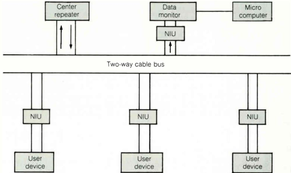
**Figure 4: NIU block diagram**
