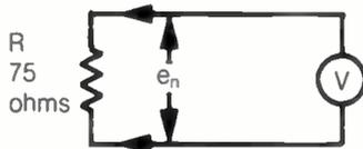
If, as in Figure 18, a sensitive high-impedance voltmeter (which generated no noise itself) could be connected across a 75-ohm resistor (or resistive source) it would measure an open-circuit noise voltage calculated by:
