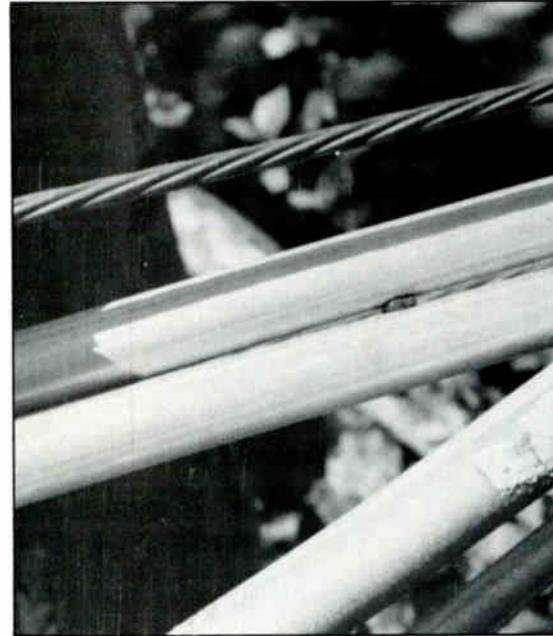
**Gnawed cable is a source of signal leakage.**
