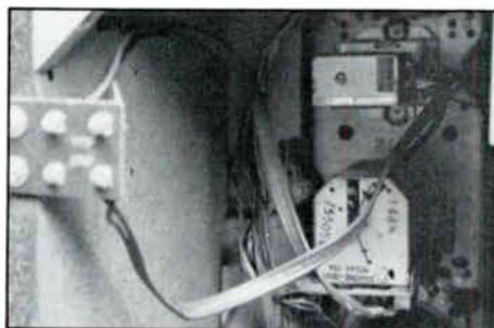
**The uncontrollable element—Internal twin lead connections in customer's television set.**
