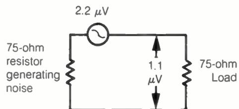
Thus the noise input into 75 ohms is 1.1 microvolts RMS, or  $-59$  dBmV. This is the basic noise level, the minimum that will exist in any part of a 75-ohm system.
