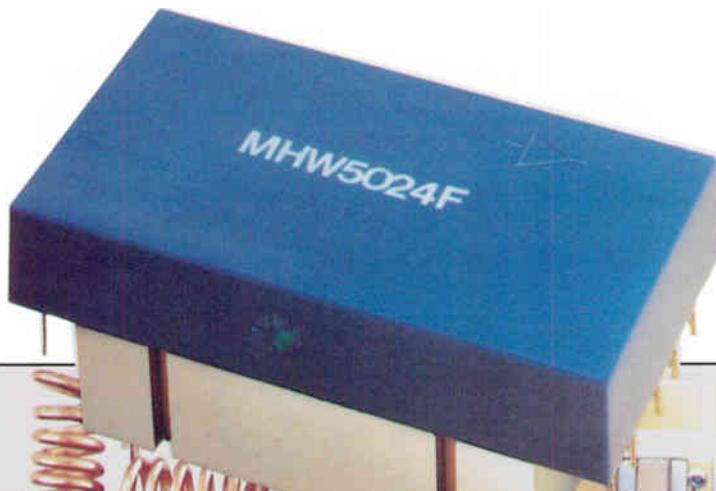
The Motorola feedforward component, Model MHW5024F, used in C-COR's feedforward amps.
