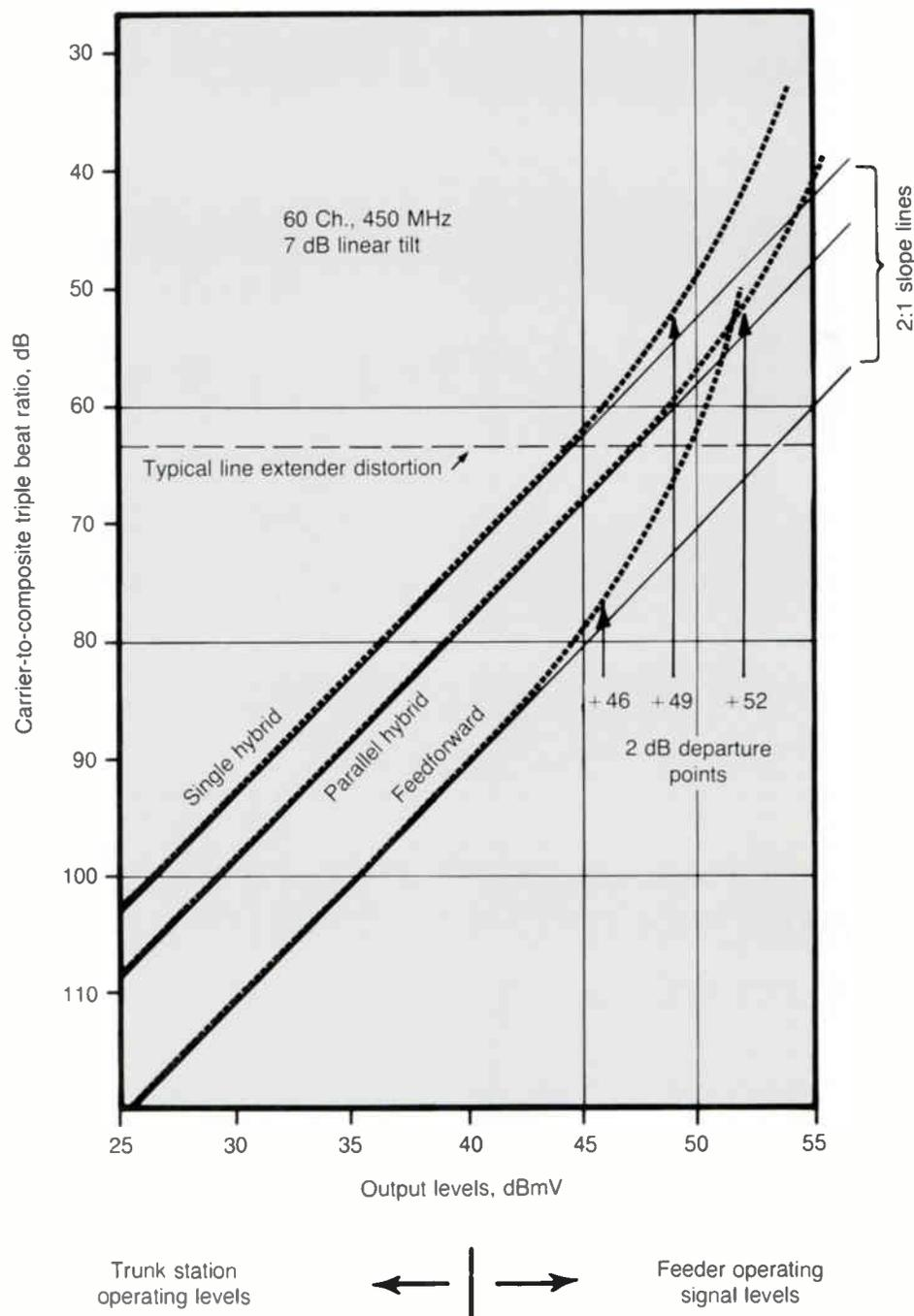
**Table 2:** Typical trunk upgrade situations using feedforward trunks
