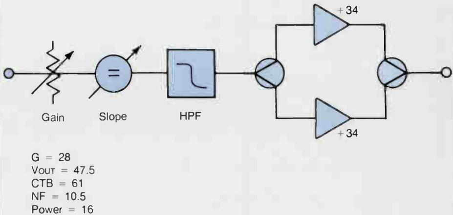
**Figure 5:** Feedforward bridger amp module
