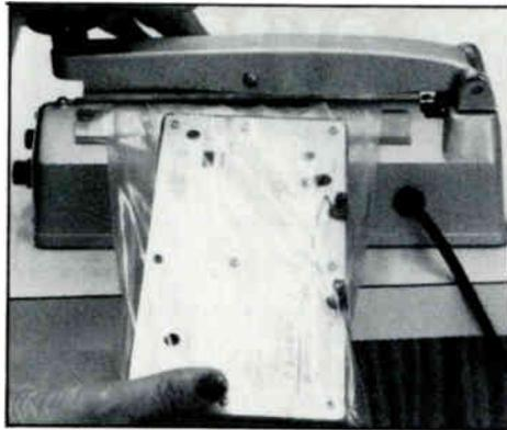
**A typical amplifier module used in many CATV systems. Advances in integrated circuitry technology plus improved amplifier design concepts can add extra channels without relocating original housings. Module modernization or replacement with improved modules may be selected for a module change out.**
