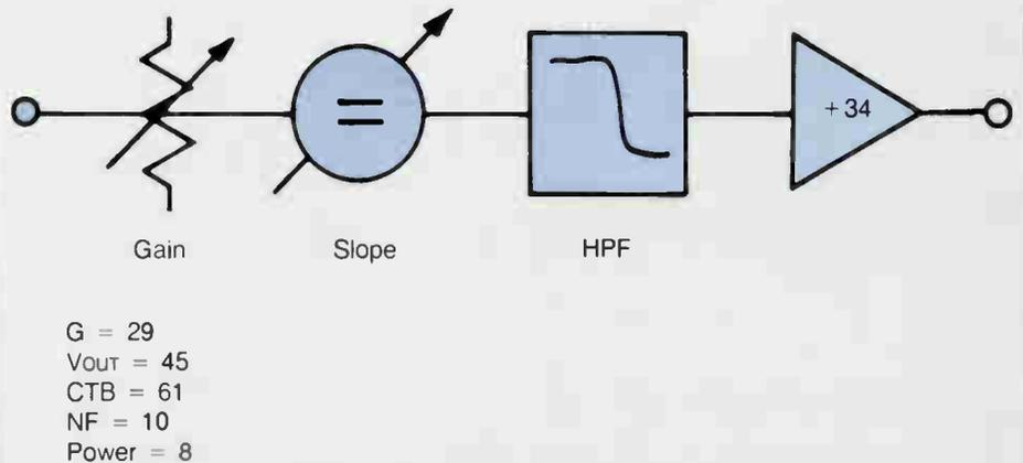
**Figure 4:** Parallel hybrid bridger amp module
