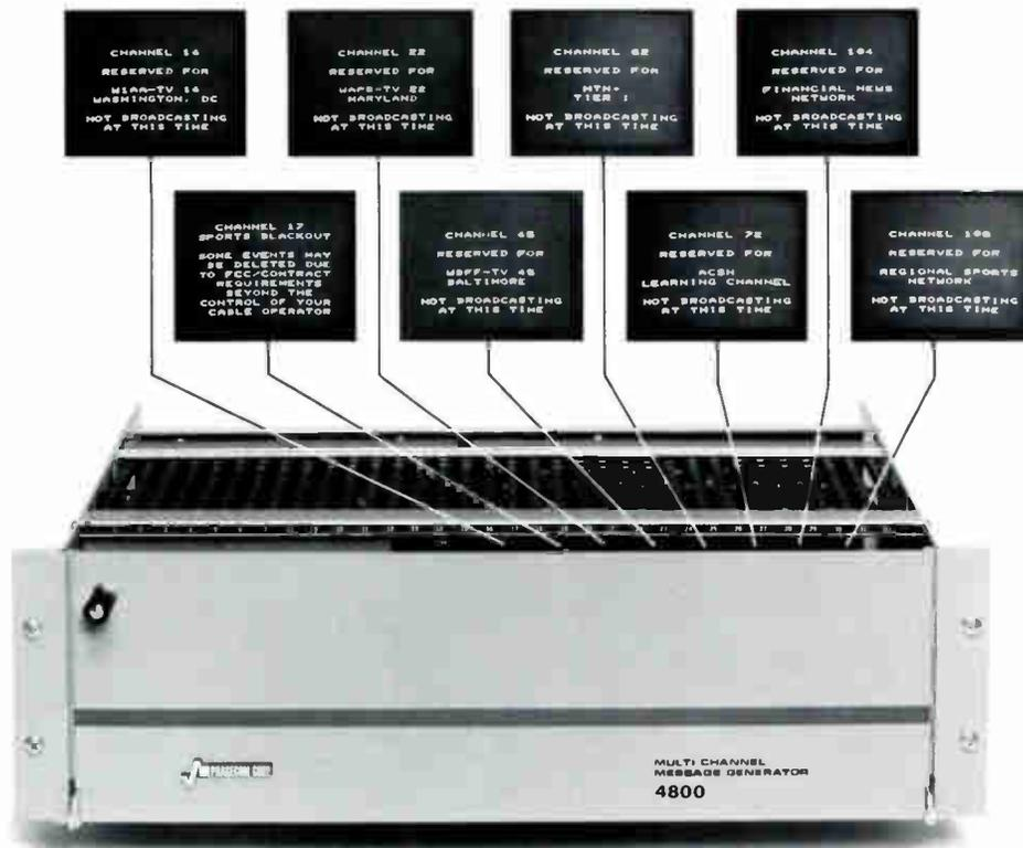
Introducing Phasecom's Model 4800 fixed character generator. It's perfect for headend operators that require fixed messages in between programming. With just one 4800, you can now accommodate up to eight channels with four different messages each. Then in the absence of program video, your pre-selected message automatically comes on the screen.
