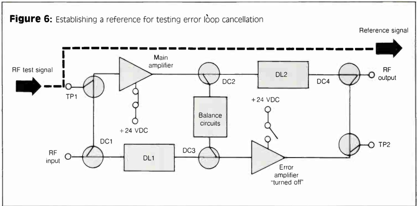
hybrids is required. For ease of alignment, the high-frequency gain of both main and error amplifiers are equal. Therefore, it is desirable to change out both hybrids upon failure of either one. However, the good device can be kept and matched with another of equal gain.
