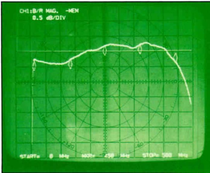
**Figure 3:** Trunk flatness with error amp failure
