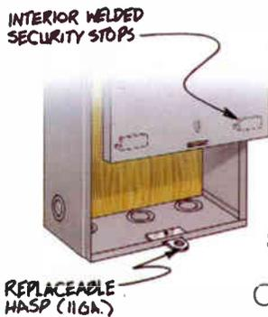
For example, CWY's all-welded enclosures are constructed of heavy 16-gauge aluminized steel—shown to outlast unpainted galvanized steel *at least five-to-one*. For added security, CWY enclosures feature security stops welded inside the front cover...a hingeless, secure cover removal system...knockouts for optional cam locks...and extra heavy-duty plated 11-gauge *replaceable* hasps.
