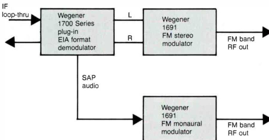
**Figure 2:** Conversion of satellite stereo sound to EIA format showing a 'dual carry' of the EIA signal plus FM band TV stereo
