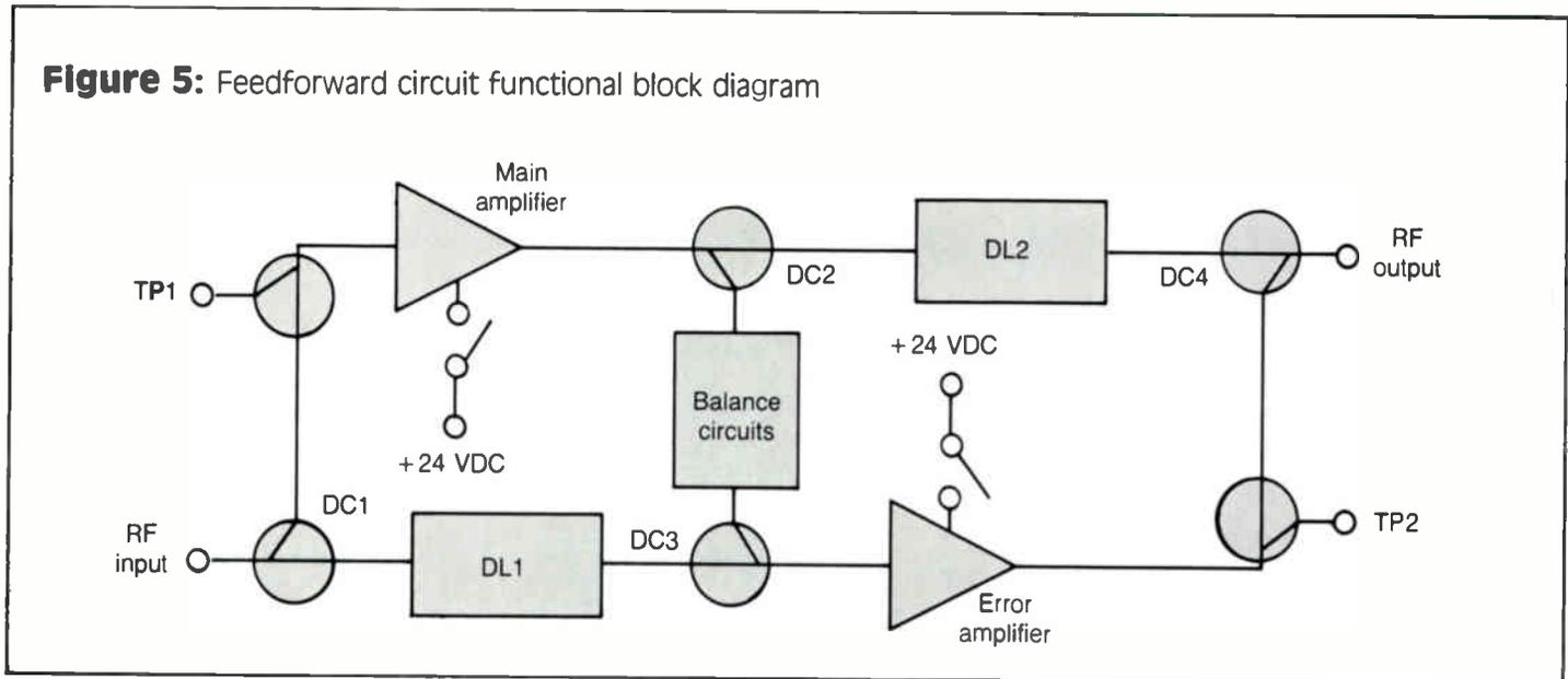
fier. The operational test consists of measuring the RF output signal level while momentarily turning off the main amplifier and then the error amplifier in the feedforward circuit. Data is transmitted to the headend where an alarm can be generated upon detection of station malfunction.
