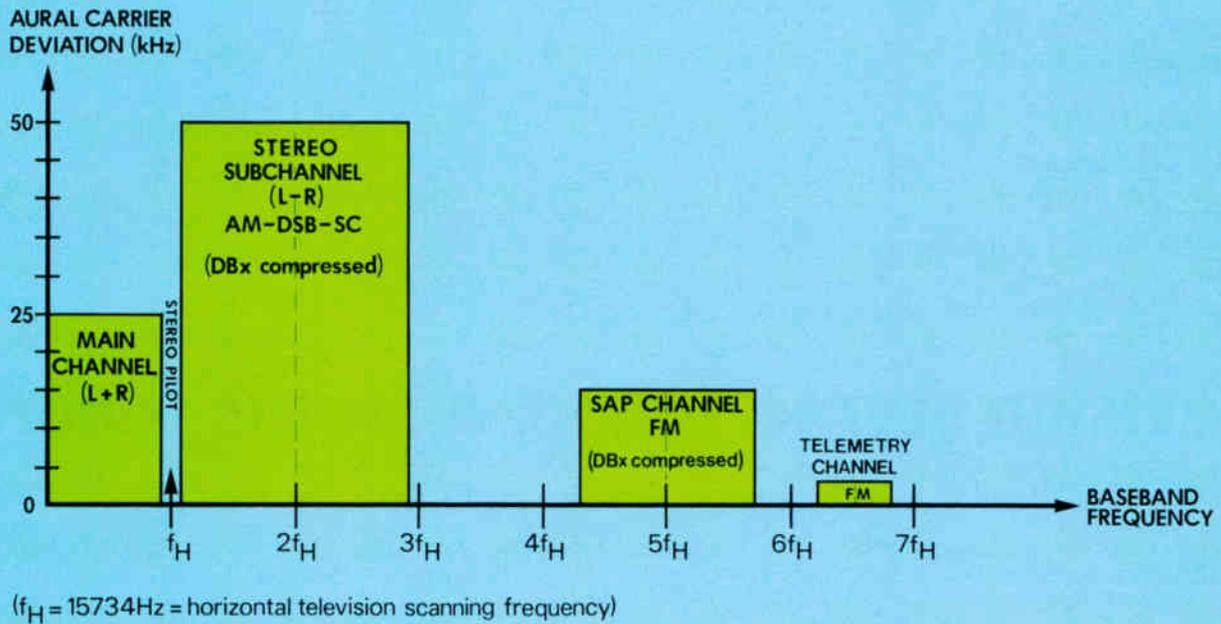
Note: Total deviation due to main and stereo subchannel modulation is limited to 50 kHz so the maximum aural deviation is 73 kHz.
