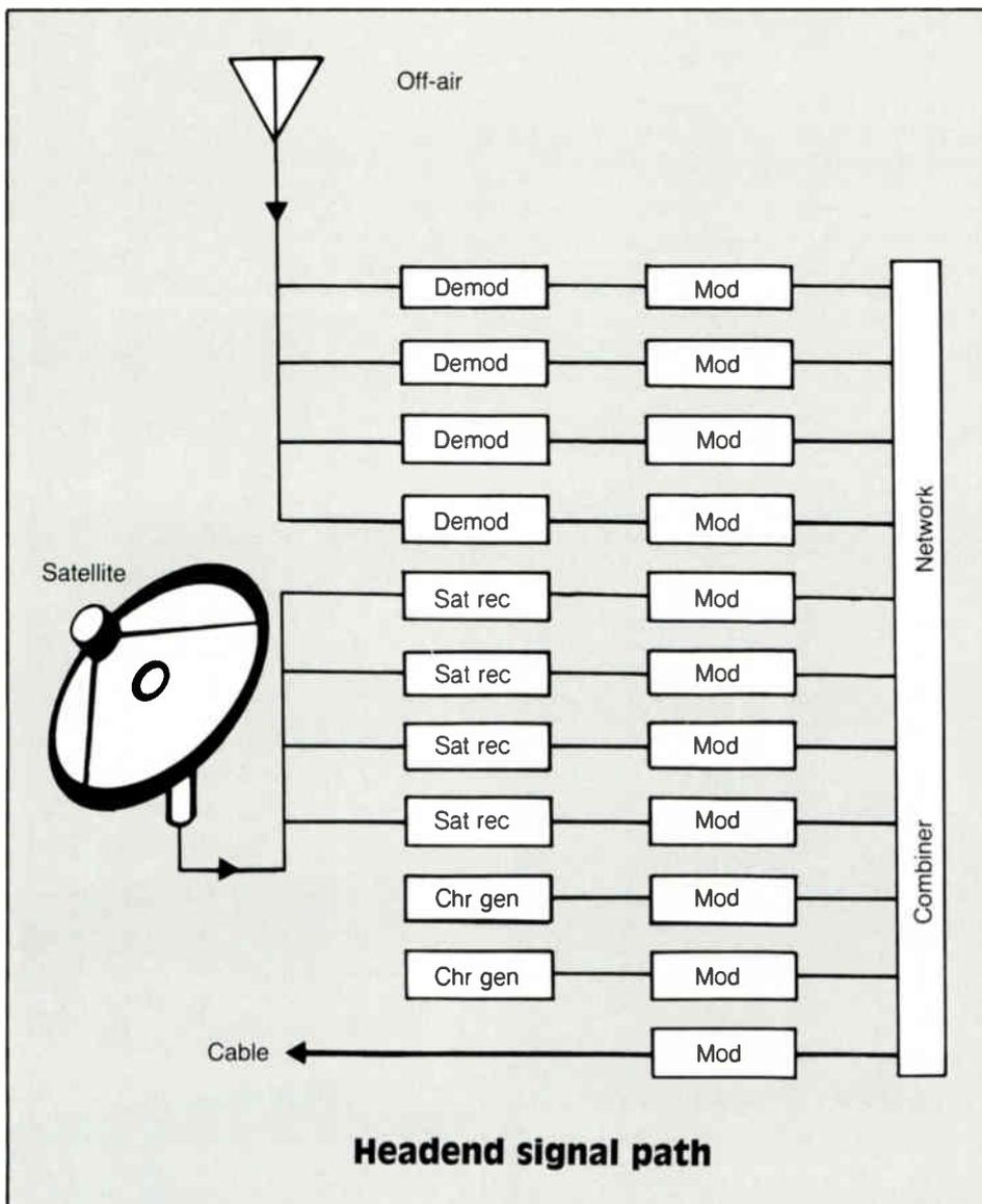
The larger system operators usually have a frequency agile modulator to act as a back-up. By having frequency agility, that is the capability to tune to any output channel, they have "spare" channels without the expense of buying another complete set of dedicated modulators.
