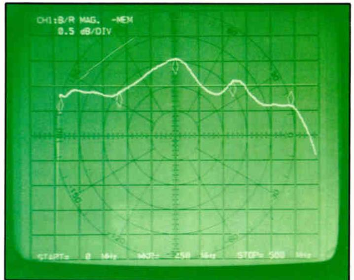
**Figure 2:** Trunk flatness with main amp failure
