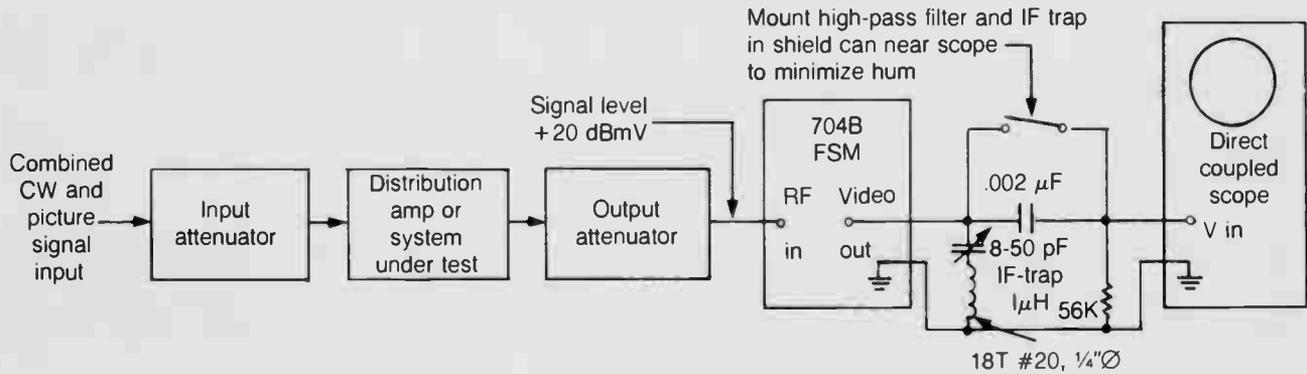
Accuracy is increased by observing the scope until a maximum of cross-modulation is seen, corresponding to the time when the interfering signal is experiencing a maximum variation.
