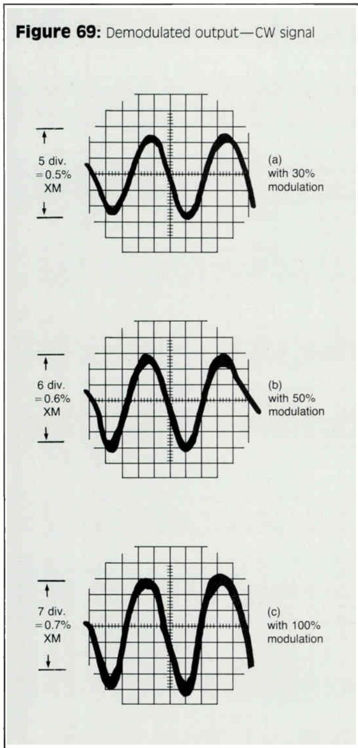
Figure 69 shows scope traces indicating the demodulated output of the FSM when tuned to the wanted (CW) signal. In each case the scope was operated in the AC mode and the gain increased so that each division corresponds to 0.1 percent cross-modulation. Applying the correction factors from Table K to each measurement gives the following result:
