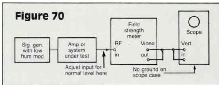
2. Set the source to a convenient frequency (the center of the band is usually a good choice), and adjust its output so the amplifier or system output is at normal level.
