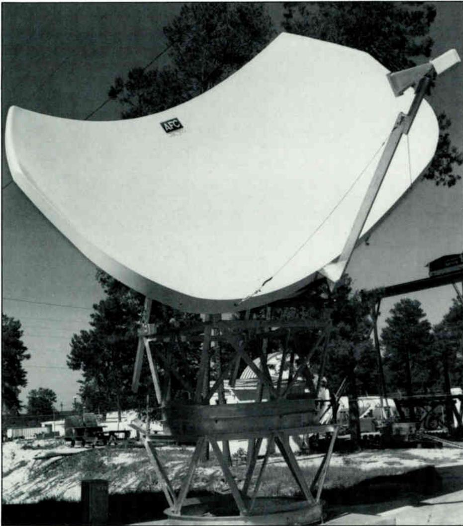
**Antennas, such as Microdyne's AFC offset-feed design, provide reduced sidelobes and an improved carrier-to-noise ratio.**
