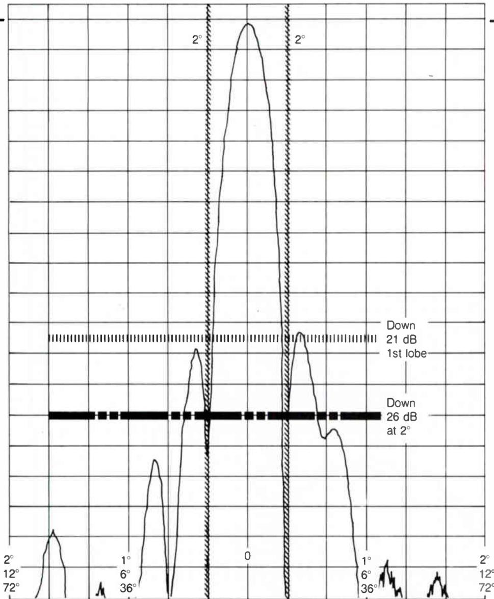
*'Be very careful to obtain and evaluate radiation patterns in the geosynchronous orbit plane . . . where the potential interference hangs out'*
