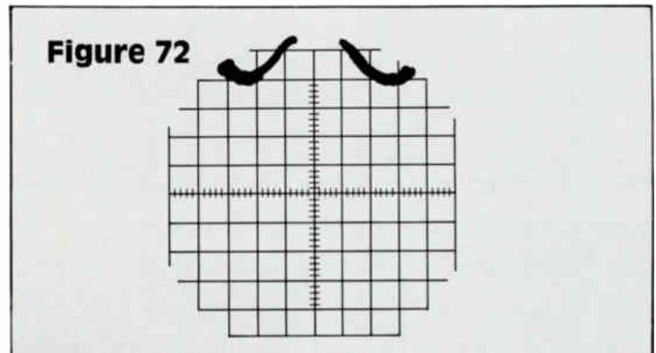
Figure 72 shows the trace with the input set for normal amplifier output, and scope gain is set so the average deflection is 10 divisions.
