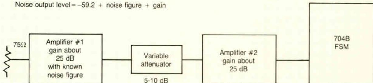
**Figure 61:** Basic test for cross-modulation
