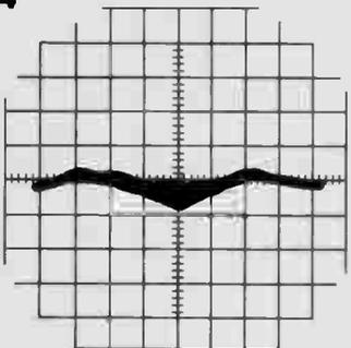
Figure 74 illustrates the hum modulation with a high-grade commercial signal generator connected directly to the input of a 704B. All of the steps have been followed, and the scope gain increased 10x, so the percent modulation indicated, with a deflection of about 0.7 div. p-p is about 0.5 x 0.7 or about 0.35 percent, which is quite good.
