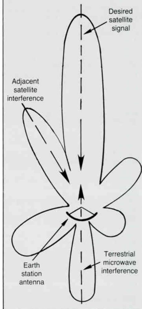
power) of each satellite. While the designed power level for adjacent satellites may be the same, one should take into consideration a potential power difference of approximately 3 dB due to such differences as age when determining the degree of interference between signals.
