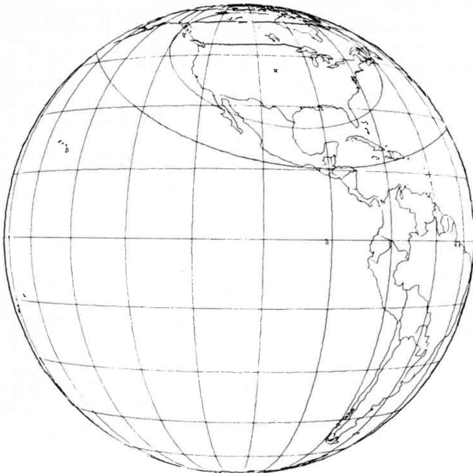
Spacecraft antenna circular cross-section beam  $-3$  dB and  $-10$  dB footprints centered near Denver. (Useful in conjunction with Figure 4 to show Az/EI versus polar mount sidelobe differences.)
