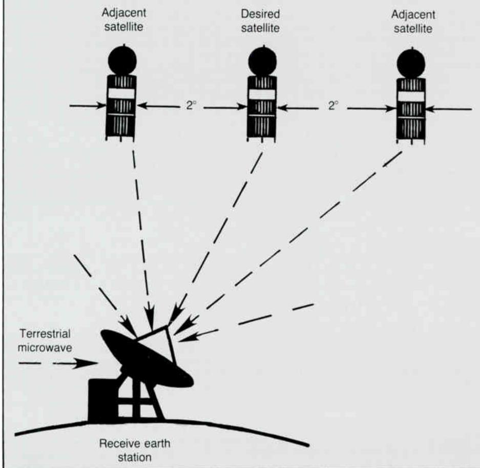
or the width of the main lobe measured at power points 3 dB down from the axis of the main lobe. However, when considering the reception of video signals for CATV or SMATV applications, it is more useful to measure the beamwidth as the angle between points at least 18 dB down from the axis.
