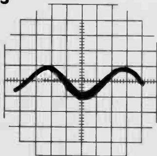
Figure 73 shows the scope trace centered, with no change in gain. The peak-to-peak deflection is two divisions, indicating modulation of 5 x 2 divisions or 10 percent. This degree of hum modulation would be excessive in an amplifier intended for CATV use; the scope trace was made while using an amplifier whose hum had been increased above normal by removing a filter capacitor.
