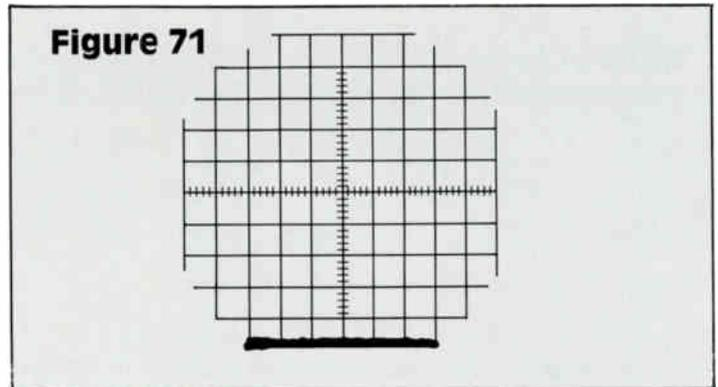
Figure 71 shows the trace at the bottom of the screen with no input to the amplifier.
