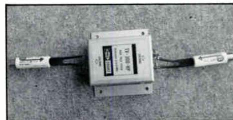
**Network used experimentally to successfully eliminate interference to VCRs from cable systems.**
