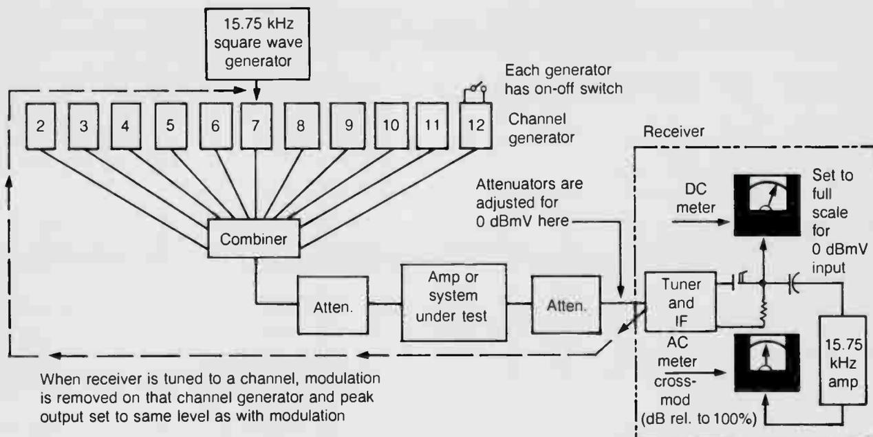
diagram of the set-up. A number of picture signals at the various channel frequencies are combined and fed through the amplifier or system under test. While viewing one of the output signals on a good television receiver, the amplifier output levels are increased, keeping the receiver input constant, until windshield wipers become just perceptible. The level at which this occurs is the maximum usable output of the system.
