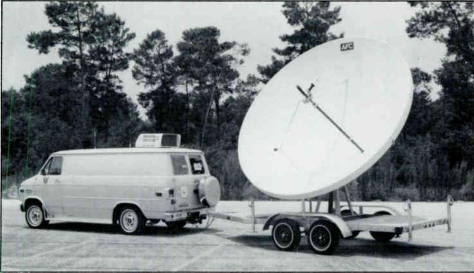
The Florida State Radio Network has successfully employed a portable system that is capable of transmitting and receiving up to four separate SCPC broadcast-grade circuits.
