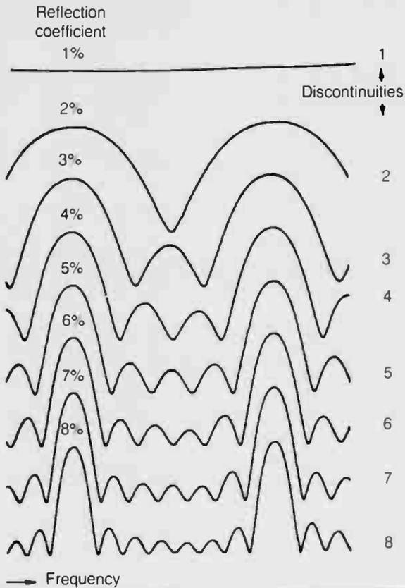
**Figure 83:** Reflection vs. frequency—three reels of CATV cable showing effects of periodicity
