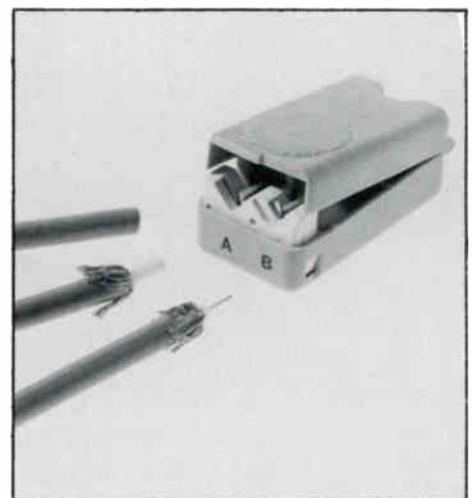
the cable itself. In addition, they can be disassembled in seconds and reused at least 25 times. Laboratory tests showed that no detectable signal degradation occurred between 40 and 1,000 MHz. The connector also withstood the application of 1,000 volts without dielectric breakdown.
