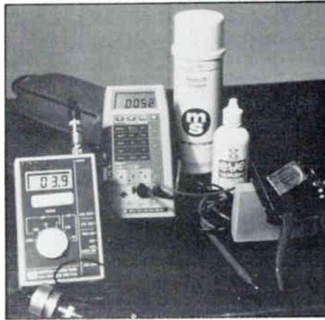
**A representative example of fiber optic maintenance equipment (l-r): optical power meter, standard digital voltmeter for test point readings, spray solvent for optical connector cleaning, eye wash (safety or first aid) and optical connector installation tool.**
