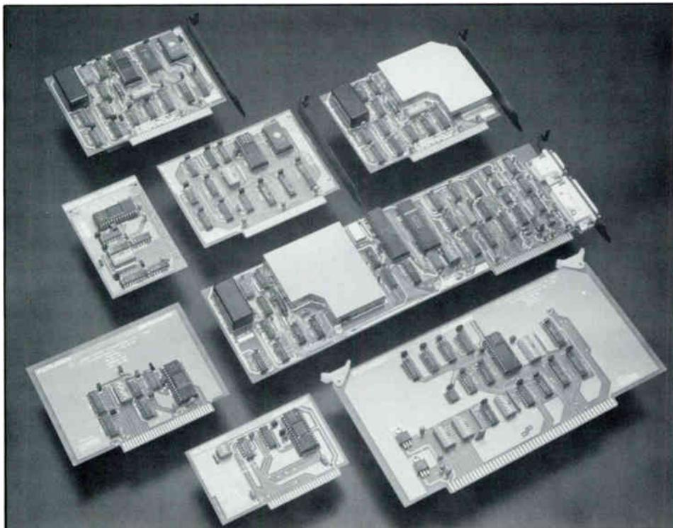
**The Encryptor™ family of data encryption/decryption boards.**
