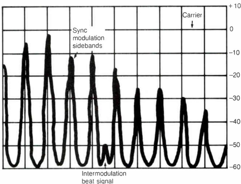
Intermodulation = carrier peak (dB) – beat signal peak (dB)
