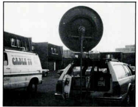
*These pictures were taken to prove that the antenna cleared the buildings and trees in front, when receiving Satcom 3-R, as well as to pinpoint the exact dish location for the proposed small earth station.*
