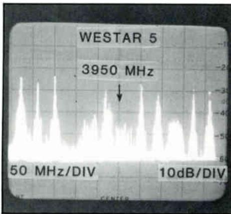
*These pictures were produced with a 4-foot diameter Prodelin dish, feeding a 63 dB gain LNA. Observe the tall Westar 5 carriers, versus the much lower amplitude Satcom 3-R signals. The view toward Satcom 3-R was somewhat limited.*
