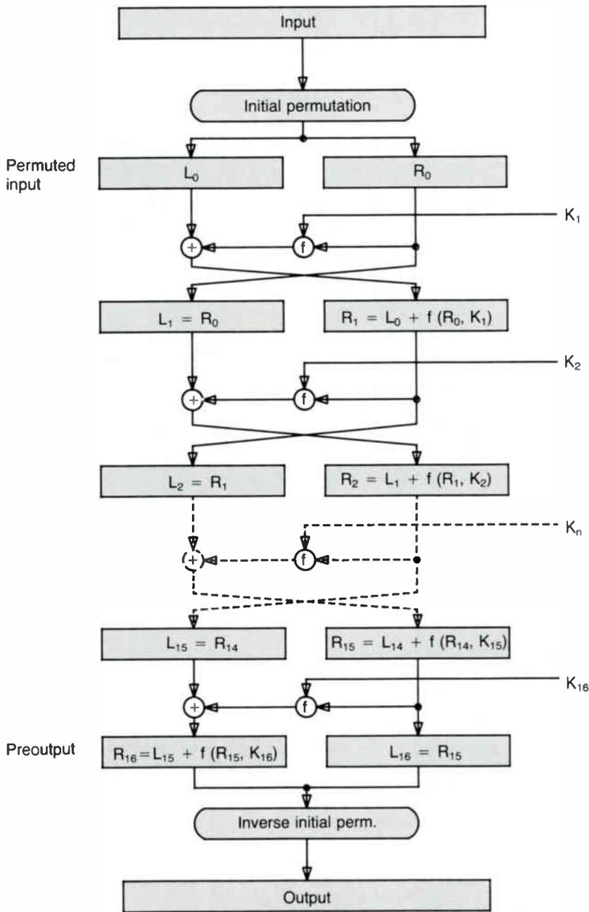
part, a number of substitutions of short sub-blocks using specially constructed substitution tables, S-boxes, and permutations of the individual bit positions. The basic DES function has been implemented by a large number of manufacturers on special-purpose large scale integrated (LSI) chips, which can encipher at megabit per second rates.
