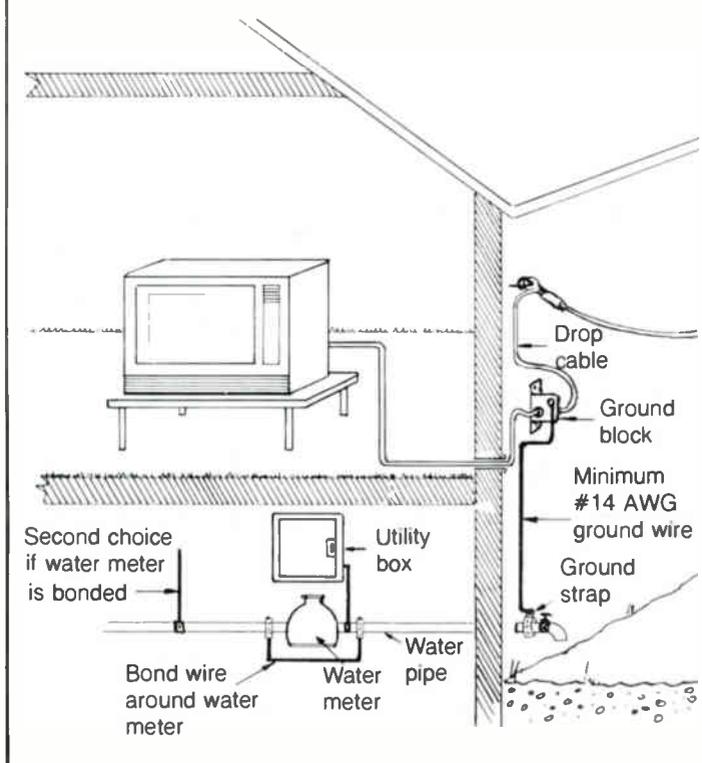
**Figure 2:** Grounding at the service conduit
