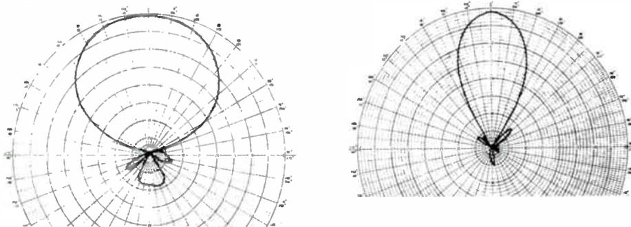
**Compare these two antenna radiation patterns. The pattern on the left side has very limited directivity. The right-side pattern is much more desirable. Also note the radiation pattern nulls at 90° and 270°.**
