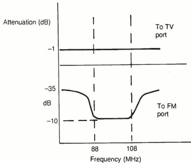
requiring an additional 3.5 dB signal. The solution was to use a frequency splitting scheme resulting in only about .5 to 1 dB signal loss to the TV set.
