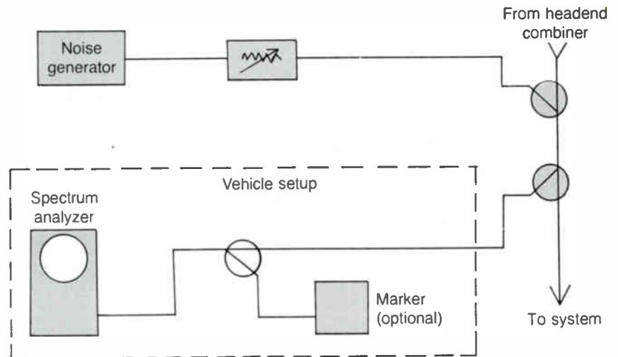
**Figure 9:** Noise response testing display
