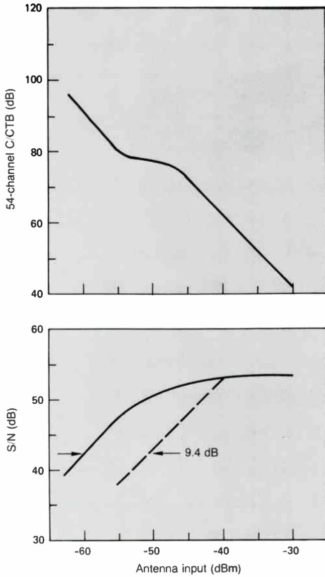
**Figure 6:** Tower-mounted LNA with AGC (5 dB waveguide loss)
