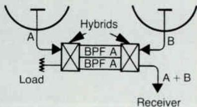
One may wish to combine (or separate) two channels. This can be done with a pair of identical bandpass filters (corresponding to one of the channels) connected between two waveguide 90 degree phase shift hybrid splitters.
