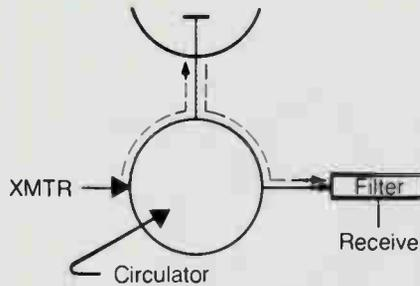
Due to antenna return loss, transmitter power may reach the receiver as shown. If the two frequencies are close, a bandstop filter is indicated, otherwise a channel bandpass filter for the receiver frequency is indicated.
