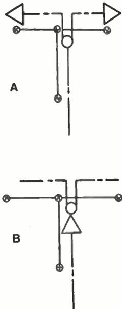
Figure 2A shows impractical designing and a waste of an amplifier. Figure 2B shows the proper placement of the amplifier in conjunction with a splitter. Note: The signal is obviously weaker in both directions in B as compared to A, however, not enough to justify the usage of an extra amplifier in most cases.
