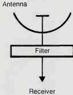
Filtering interference from off-air reception. The filter is usually a channel bandpass unless interference is adjacent channel. Then a bandstop is usually more economical. If two or more channels are received from the same antenna, the bandpass filter is correspondingly wider.
