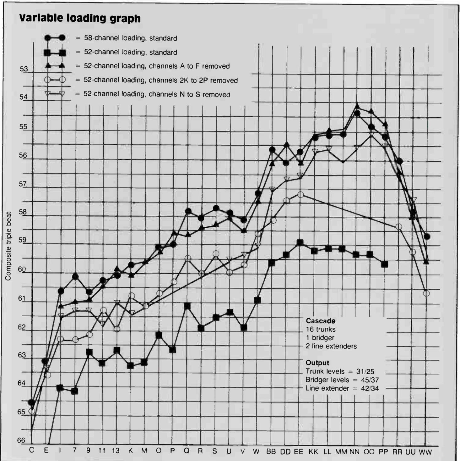
tests have shown that channels in this frequency spectrum do not have a meaningful impact on the overall beat power distribution.
