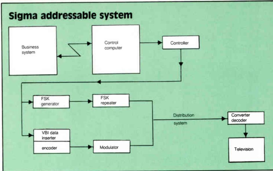
thentication information is delivered on the frequency shift keying (FSK) control channel, at 104.75 or 112.7 MHz. The control channel communicates information to both encoders and decoders. Control information must match the VBI data, creating a lock that prevents the decoder from being defeated by feeding it false information.
