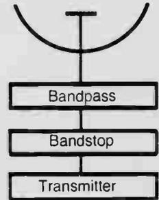
A wide band (multi-channel) transmitter usually requires a bandpass filter to suppress the spurious (out of band) emissions which are usually present. Because of the wide passband, the bandpass may not be sufficiently selective to suppress emissions at frequencies immediately below the first and above the last channel transmitted. Hence separate bandstop filter may also be needed.
