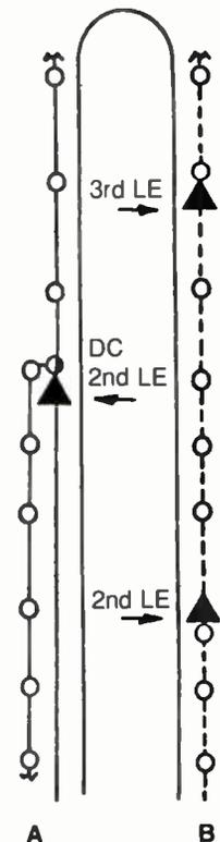
Figure 3B shows straight line placement of taps and an unwanted third line extender. Figure 3A shows elimination of the third line extender by eliminating the taps as shown and pushing the location of the line extender forward, utilizing the backfeed.
