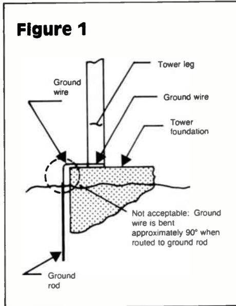
time and trouble to correct the grounding on all your towers, because it will greatly reduce the chances of damage to equipment when lightning strikes.
