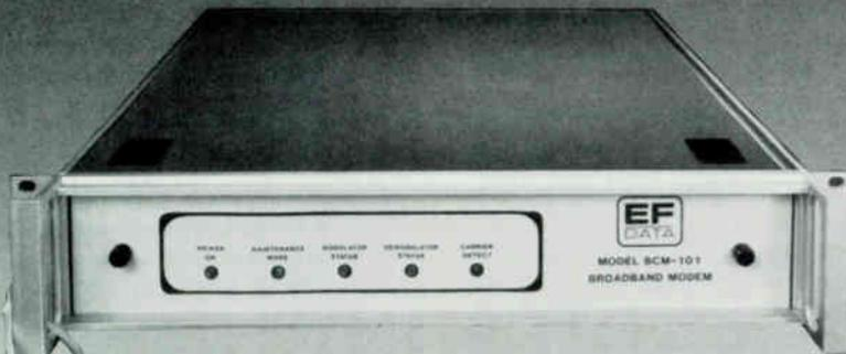
Microphonics, vibration, synthesizer and cable noise are problems of the past with EF Data's BCM-101 Broadband Modem. A new proprietary technique using digital signal processing makes the modem tolerant to system noise and cable intermodulation products. We call it EFplex and it puts our BCM-101 light years ahead of the competition as a totally error-free product for data transmission.
