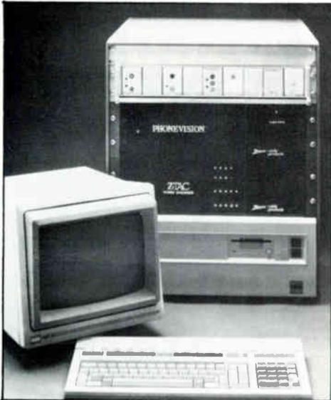
**Zenith's Phonevision is built around a new CATV headend hardware and software system that can process more than 1,000 program orders per minute.**
