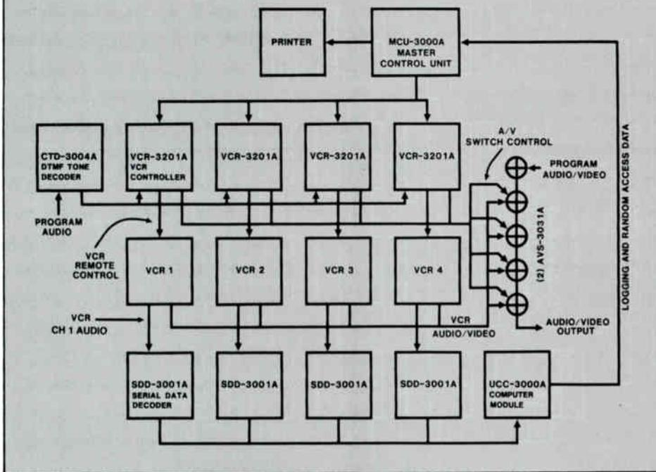
block diagram of a multiple-VCR random-access system.
