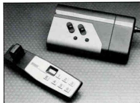
**The Shuttle Communicator can be used with encryption devices, such as the Enigma Logic Safeword system.**
