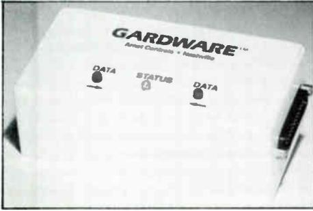
into the computer before protected software will operate or protected on-line systems can be accessed. When the connection is made, the protected software or on-line system and the Gardware security module form a "lock and key" that only will function in unison. The
