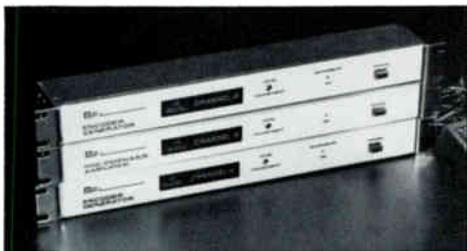
Model LS-(channel) lower adjacent security module, an optional accessory, is used when the lower adjacent channel is unoccupied by programming. It generates an RF signal at the lower adjacent sound frequency making it impossible for subscribers to fine-tune in part of the premium programming.
