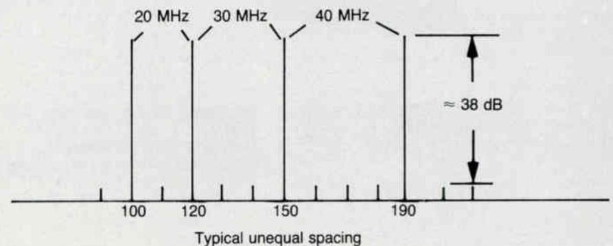
**Figure 7:** Typical second order intermodulation distortion
