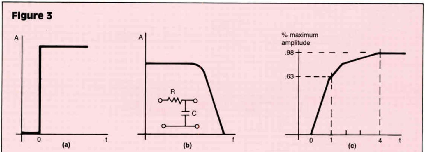
There is another effect that must be considered. When a steep wavefront, such as a leading edge of a single pulse (Figure 3a), is introduced into a narrowband filter (like a radio receiver) the output wavefront is not as steep since it takes a finite time for the signal to build up and reach its peak value within the narrow bandwidth.
