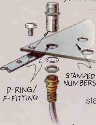
panels are labeled permanently by stamped numbers on the tops of the panels. Once leads are connected, they need never be touched again—checking or changing status means handling only jumper
