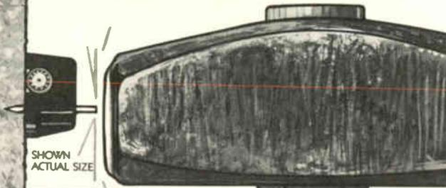
**ONETAP™ CLIP fastens coax cable to poured concrete — no need for special tools!** Tempered steel pin easily penetrates poured concrete, cinder blocks, mortar, bricks, hardwood floors. Strain relief grip holds ONETAP™ CLIP on cable while pin is driven — route cable as you install. 3 sizes fit all coax cable installs. Patent Pending.
