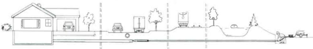
Pierce Arrow™ pneumatic underground piercing tools penetrate rocks, small boulders and tree roots, making a straight compacted hole for pipe or cable. They eliminate the added work of open trenching.
