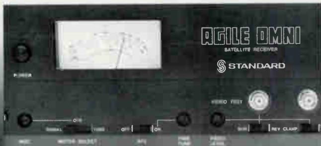
Operating functions including MGC, AGC, AEC, level sets, normal/invert video, clamp/unclamp video, skew, subcarrier frequency selection, video, and IF test points are conveniently located on the front panel. Meter reads C/N ratio, signal strength, or center tune.
