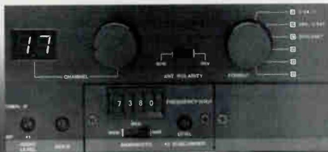
Format control enable selections of desired satellite system. Direct-reading channel selector displays transponder-assigned channel. Second selectable subcarrier and space for optional third subcarrier or descrambler modules.
