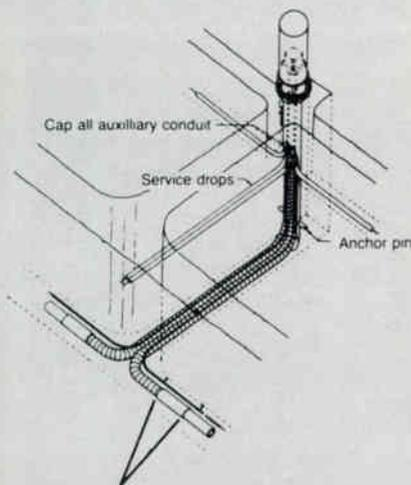
Note: When conduit changes direction, splice with flexible conduit to semirigid and make all turns with flexible conduit or appropriate conduit sweeps.
