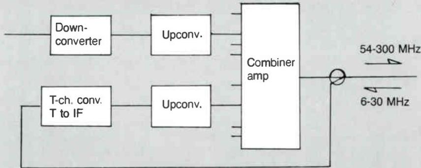
The concept of "cherry-picking" the cable system channels and eliminating converters led to packaging SCS in 12-channel increments. However, the SCS cabinet can accommodate up to 18 channels with space remaining for additional equipment. Fundamentally, SCS is similar to most top-line heterodyne headends (Figure 1), including its many options for special situations.
