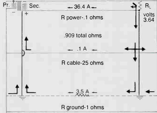
**Figure 14: Power bonded to earth ground and cable**
