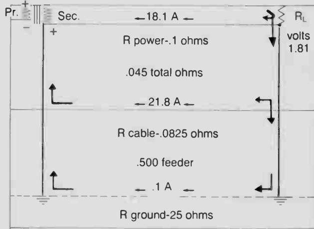
**Figure 8:** Power bonded to earth ground and cable
