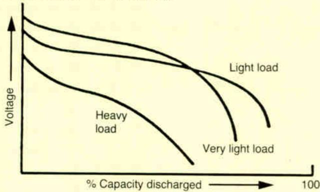
**Figure 4: Discharge curves at hourly intervals**
