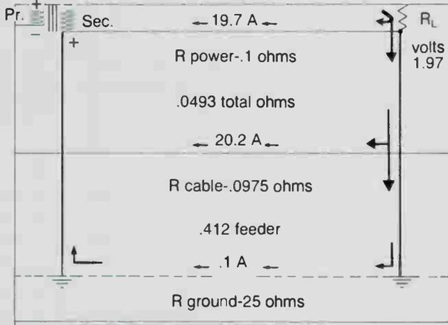
**Figure 7:** Power bonded to earth ground and cable
