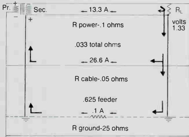
**Figure 9:** Power bonded to earth ground and cable
