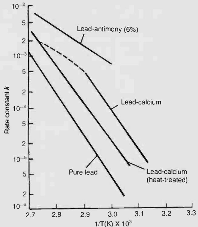
Corrosion rate constant  $k$  on log scale vs.  $1/T(K)$  for different lead-alloy grids.
