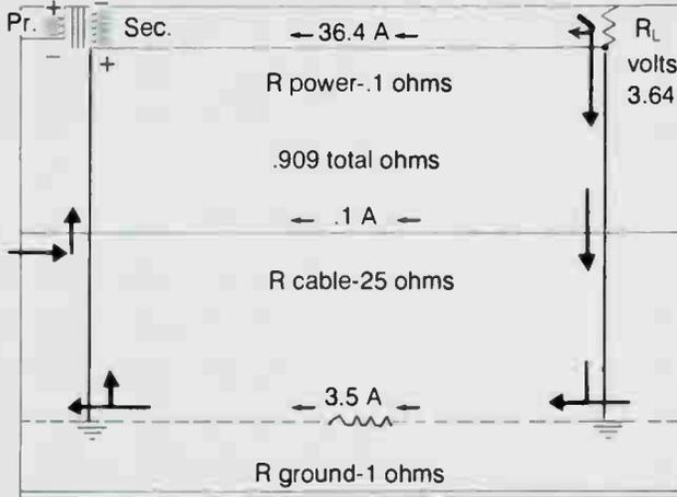
**Figure 15: Primary bonded directly to secondary**
