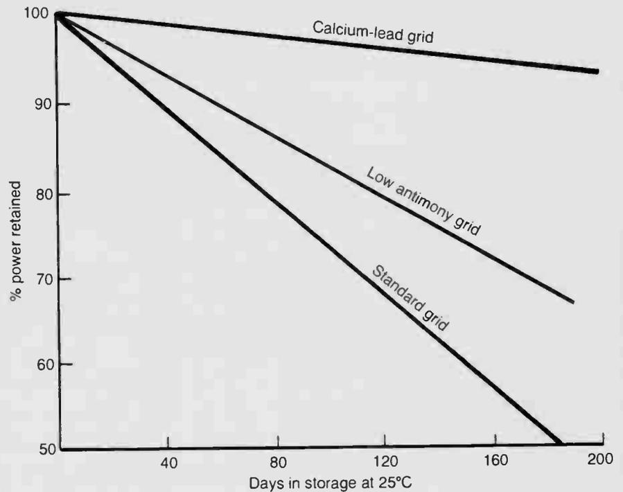
**Figure 2: Plate corrosion rate chart**
