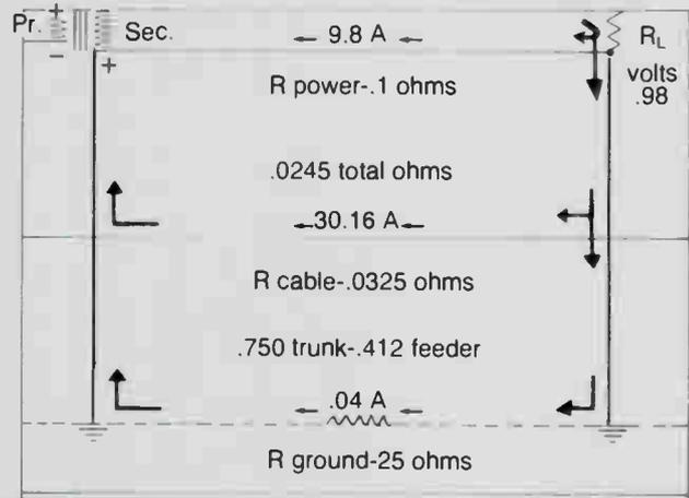
**Figure 11:** Power bonded to earth ground and cable
