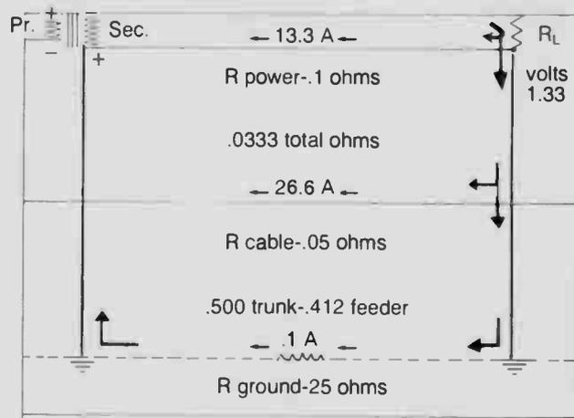
**Figure 10:** Power bonded to earth ground and cable
