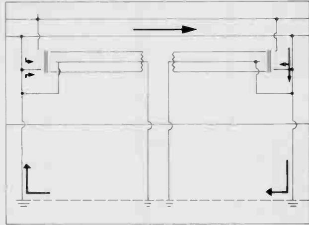
**Figure 16: Primary and secondary bonded to cable**
