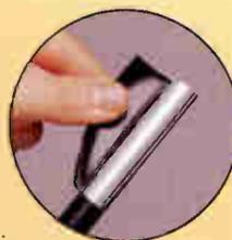
Jacket bonded to sheath for additional handling ease and increased corrosion protection. Peels away easily, leaving no adhesive residue. Continuous conductor-through-jacket bonding greatly increases sidewall and pull strength. Extra-rugged LLDPE\* jacket dramatically increases abrasion resistance and reduces pulling friction.
