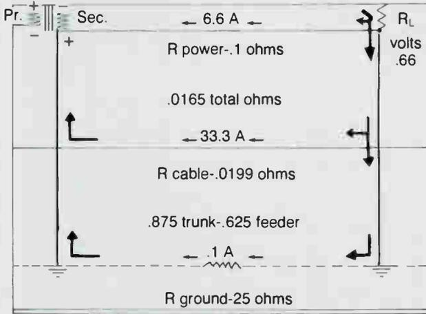
**Figure 13: Power bonded to earth ground and cable**
