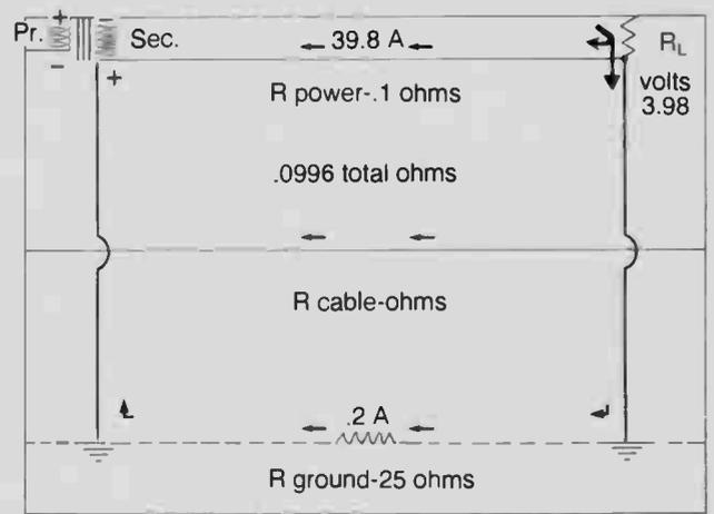
**Figure 5:** Power bonded to earth ground
