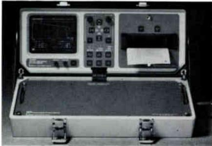
singlemode or multimode, the TD-9950 offers plug-in 850, 1300, 1550, and dual wavelength 1300/1550nm modules. The TD-9950 combines high performance with user-friendly software and built-in digital X-Y plotter for easier, faster characterization of fiber optic cable links.
