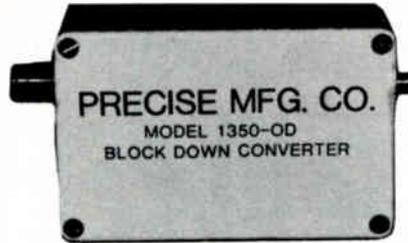
The PRECISE Model 1350-OD, Outdoor Downconverter is designed to be used with an LNA to provide a 270 - 770 MHz block down conversion of the 3.7 - 4.2 GHz satellite TVRO signal.
