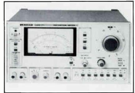
of less than 1 percent THD, this instrument will complete the measurement, eliminating almost all manual tuning. It also features S/N measurement and AC signal level measurement capabilities.
