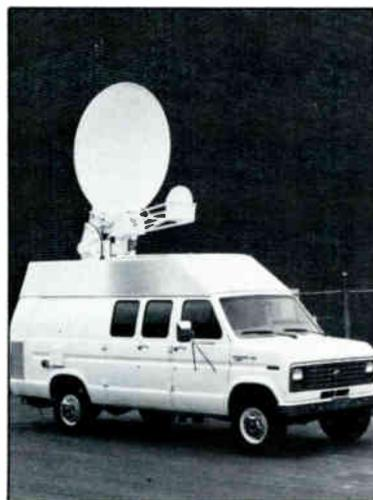
The offset VSAT mobile antenna.
