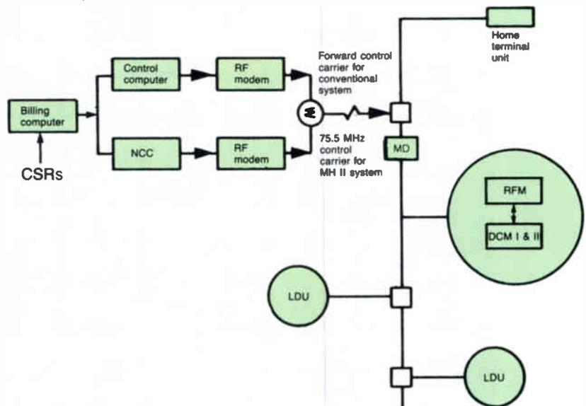
**Figure 2:** Headend control system with a common control computer
