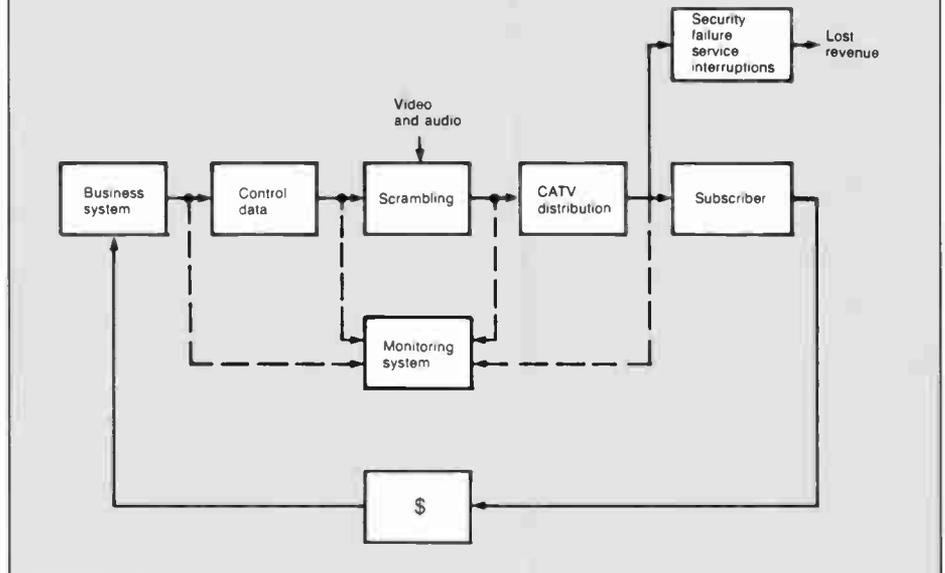
upon command is a fundamental requirement of an addressable system. Thus, control over the descrambling decoder is the control data
