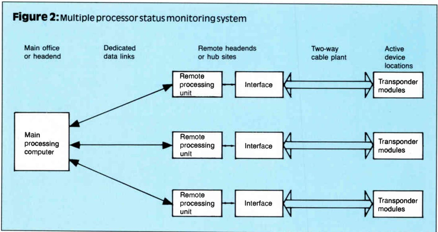
ing and controlling a number of functions. Table 1 highlights many of the monitoring and controlling features available. These capabilities can provide a cable operator with tremendous flexibility, and a well-planned status monitoring system actually will help to reduce plant maintenance costs. A cable operator can monitor the operational status of the entire cable system, immediately identify and locate problems, and remotely
