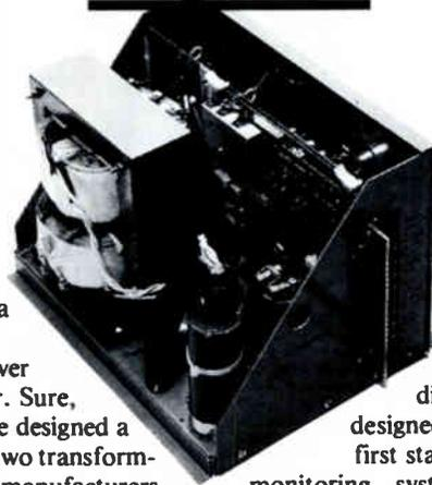
Pull off our cover and see why Alpha is the CATV Stand-by Power Supply leader. Sure, we could have designed a system using two transformers like most manufacturers, but no, we decided that a single ferro-transformer would be more reliable. It was gutsy, it was innovative, and it works.
