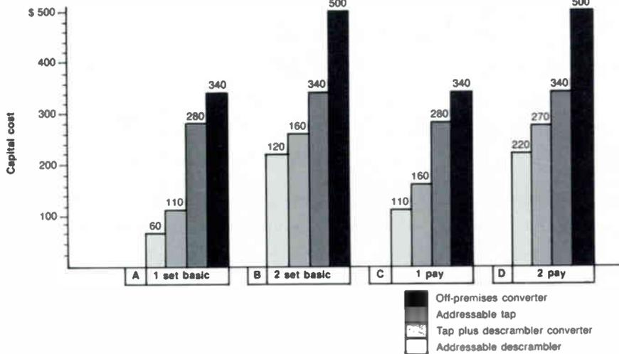
combination of a limited-function addressable tap with addressable descramblers for pay service can have advantages in both operating cost and security. In this system (Figure 4), access to all programming is secured via addressable tap.
