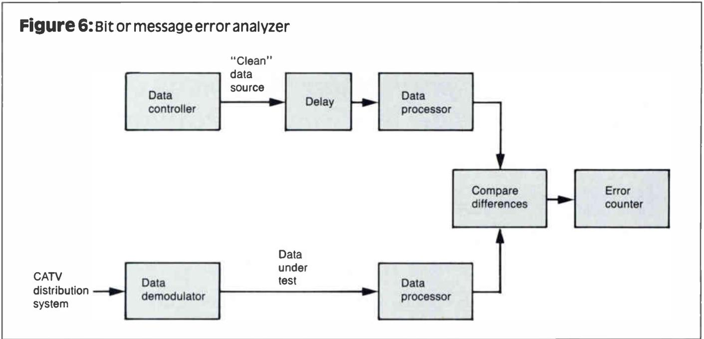
some bit errors. A particular system bit error counter may show six bit errors in a one-minute time period or 0.1 errors per second. If the data transmission rate is 10,000 bits per second there is one error for every 100,000 bits, and the BER is expressed as  $1 \times 10^{-5}$ .
