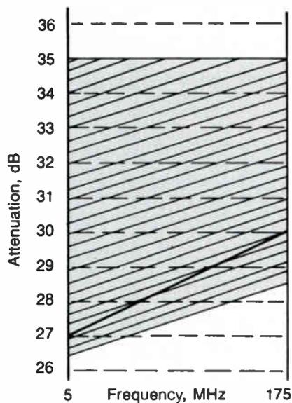
\* Using standard CATV taps, +45 dBmV amplifier output, standard in-line equalizer.
