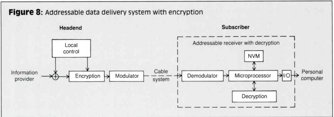
cess to the data. Unfortunately, the receiver needs to know the key that was used in the transmitter so it can decrypt the data. So, keys must be sent down the cable to the appropriate receivers. The keys must be encrypted using keys known by both the transmitter and receiver. They should be changed as often as practical.
