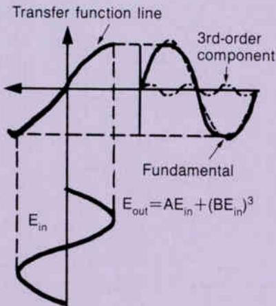
**Figure 7:** Third-order harmonic distortion (frequency domain)
