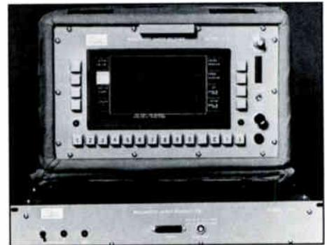
then set up specific guard bands around the carriers to protect them from any sweep interference. The receiver reads both the sweep and carrier levels, integrating them to create a high-resolution (better than 0.25 dB) sweep response.
