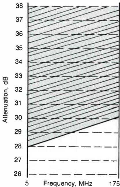
\* Using standard CATV taps, +48 dBmV amplifier output, standard in-line equalizer.
