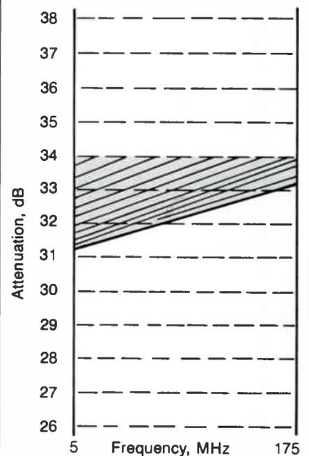
\* Using split-band taps, +48 dBmV amplifier output, standard in-line equalizer.
