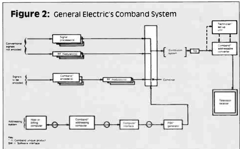
system), which processes and off-loads the proper addressing codes to the system controller in the headend. If the billing system is located outside the headend, then the communication link is provided by modems.
