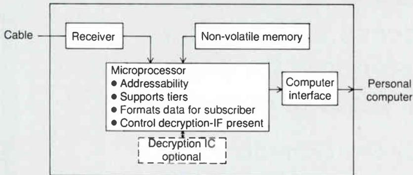
amount of control information to a minimum. Control information gives the cable operator control and flexibility, but has no benefit to the subscriber. In fact, it reduces the amount of information he can receive. The amount of control information can be minimized by carefully studying what control is necessary and by using both individually addressed and global commands to the data receiver.
