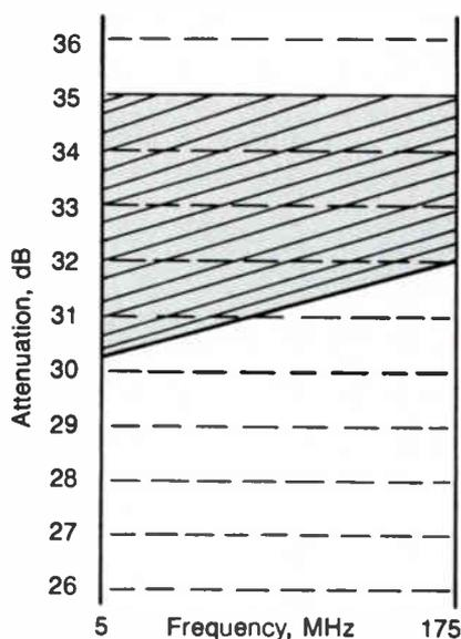
\* Using standard CATV taps, +45 dBmV amplifier output, padded in-line equalizer.
