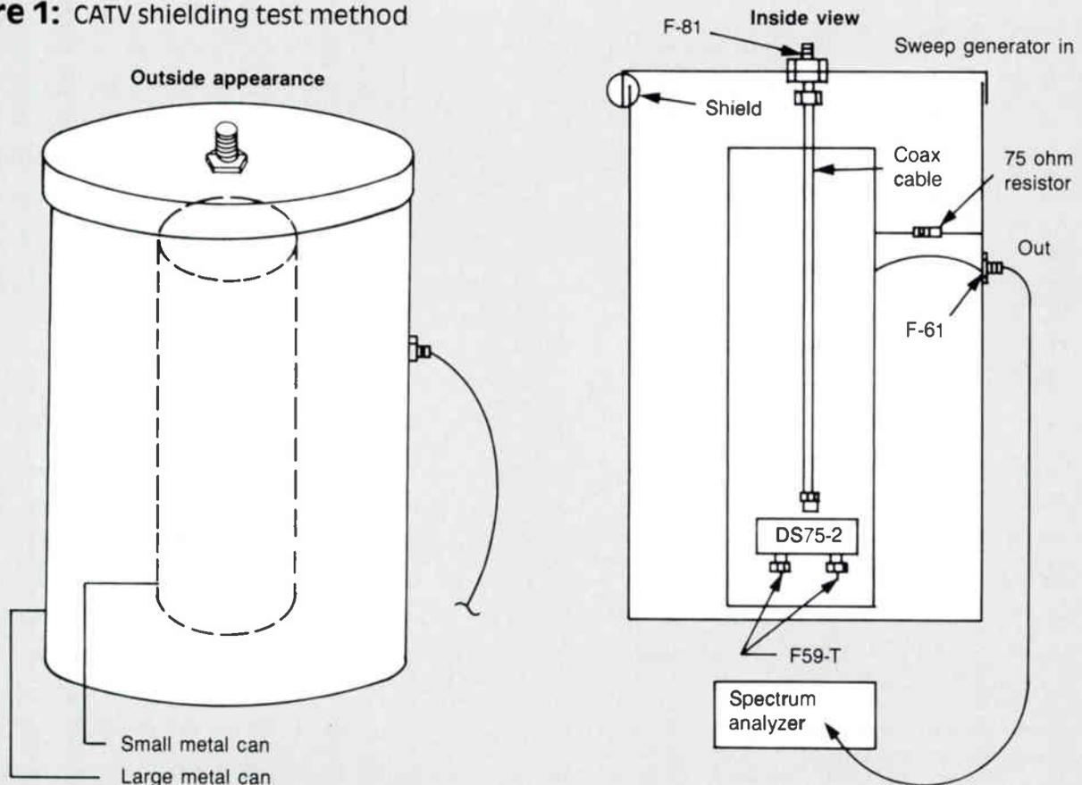
**Figure 2:** Concentric chamber shielding method
