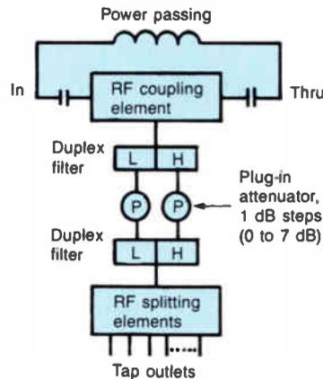
**Figure 3: Feeder design using split-band tap units**
