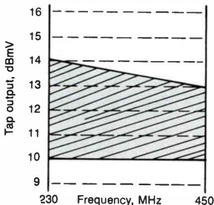
**Figure 11: Forward tap window, split-band taps**
