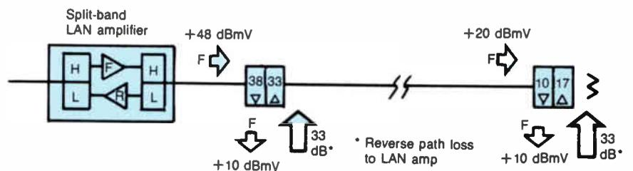
Lower amplifier output levels require lower value taps, thus reducing the maximum reverse path loss. In addition, the end of feeder is limited. The amount of coaxial cable used between amplifiers or from an amp to an end-of-line tap is specified so that the minimum path loss is increased. Both of these actions result in higher installation cost, increased use of costly actives and a marginal improvement in the performance of the system vis-a-vis return path loss variations.
