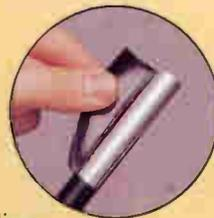
Jacket bonded to sheath for additional handling ease and increased corrosion protection. Peels away easily, leaving no adhesive residue. Continuous conductor-through-jacket bonding greatly increases sidewall and pull strength. Extra-rugged LLDPE\* jacket dramatically increases abrasion resistance and reduces pulling friction.
