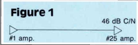
dBmV input instead of the typical 20 dBmV. With an NF of 10 dB the C/N will be:  $59 - 10 + 17 = 66$  dB C/N (line extender). We now use Formula 3 to combine the different C/N ratios:
