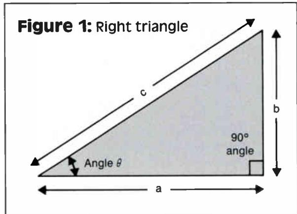
From these ratios, formulas can be derived (Figure 2) to determine solutions to problems that occasionally crop up in CATV engineering. Examples of the application of some of these formulas are on the next page.
