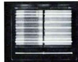
variable knob fully counterclockwise (red light off); sweep pushbutton 2H in; response to "FLAT"; sync on "INT"; DC restorer on; line selector off.
