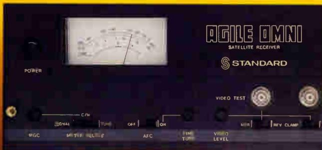
Operating functions including MGC, AGC, AFC, level sets, normal/invert video, clamp/unclamp video, skew, subcarrier frequency selection, video and IF test points are conveniently located on the front panel. Meter reads C/N ratio, signal strength or center-tune.
