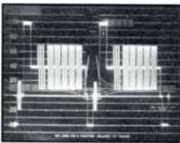
**Figure 4: Two lines with .25 H/cm display**
