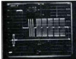
**Figure 14:** VITS signal of field one
