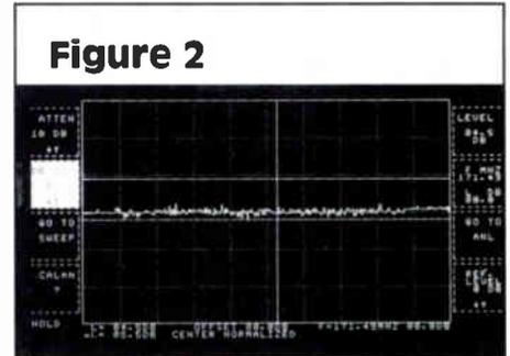
for that high channel's continuous noise. The mid-band signature, with its 20 MHz wide "hump" of noise explained the random background noise that seemed to always be there throughout the band.
