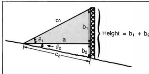
To calculate the height of the tower in this situation, first measure  $c_2$  with an accurate measuring wheel; also measure angle  $\theta_2$  from level down to the base of the tower, and angle  $\theta_1$  from level up to the top of the tower. (Assume  $c_2 = 200$  feet,  $\theta_2 = 8^\circ$ , and  $\theta_1 = 25^\circ$  for this example.)
