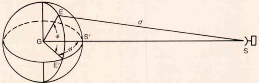
**Figure 2:** Earth station E and local horizon (elevation angle  $\theta$ )
