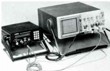
Calibration Mode: Standard on all models—The calibration mode enables the user to set up the DTDR to test cable types with different dielectric characteristics (nominal velocity of propagation). Any known velocity of propagation speed can be entered in the "Set" position using the Keypad.
