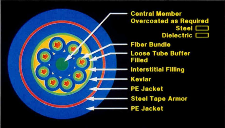
**Cross section of a fiber-optic cable**
