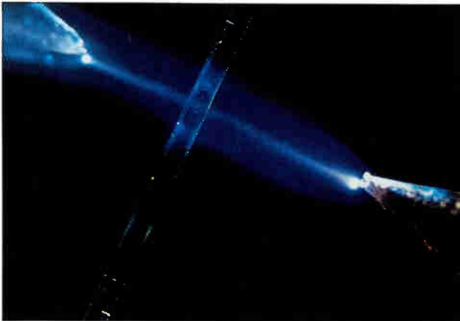
The electric arc of a fusion splicing machine heats the intersection of two fibers to the point where they flow together to form a single integral piece.
