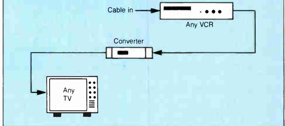
**Figure 2:** Hookup with converter in front of VCR
