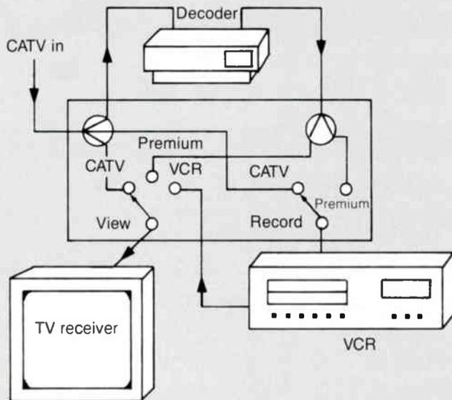
**Figure 5: Ganged RF switches**
