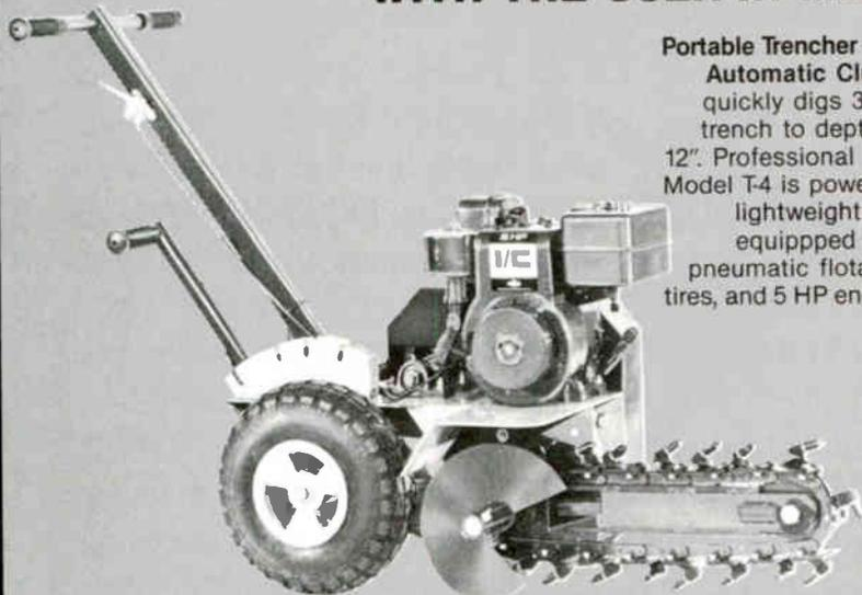
Portable Trencher with Automatic Clutch quickly digs 3-1/2" trench to depth of 12". Professional type Model T-4 is powerful, lightweight and equipped with pneumatic flotation tires, and 5 HP engine.
