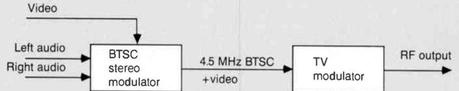
**Figure 8: 4.5 MHz BTSC and separate baseband video interface**
