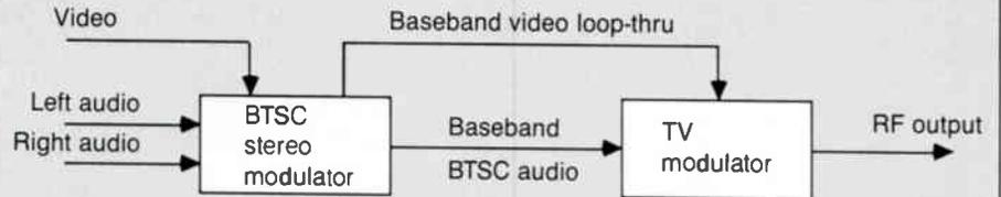
**Figure 7: 4.5 MHz composite video interface**
