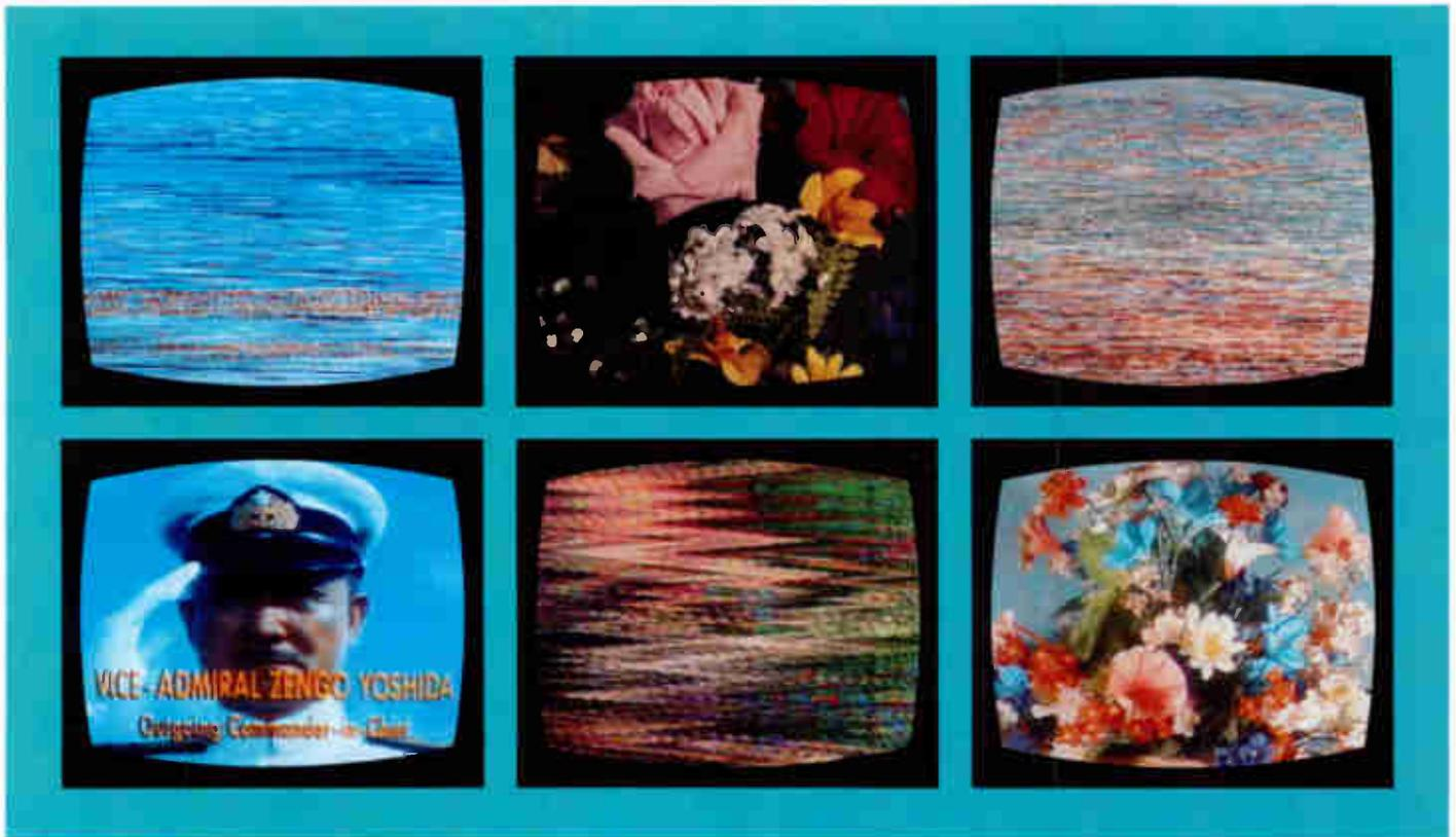
Encryption using line dicing/rotation. Scientific-Atlanta's B-MAC encryption. Example of encryption using line shuffling.
