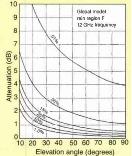
rain rate or elevation angle is less favorable, the critical design factor for dish size might be availability.
