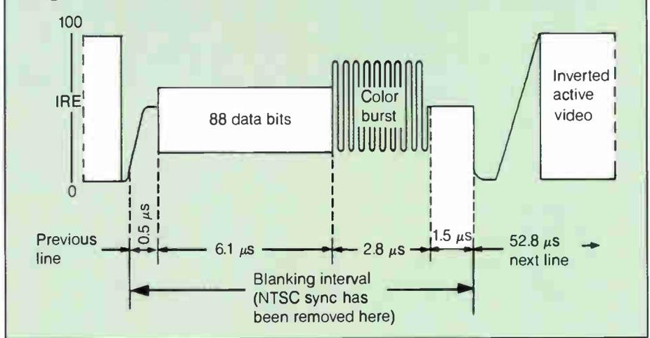
one line than on the preceding line. This either advances or delays the start of each line, producing a slewing of the individual lines. No data is omitted, it merely is sent in advance or saved for later. It is this sequence of advance/delays that is encrypted and as before, the encryption/decryption algorithms can handle this rate.
