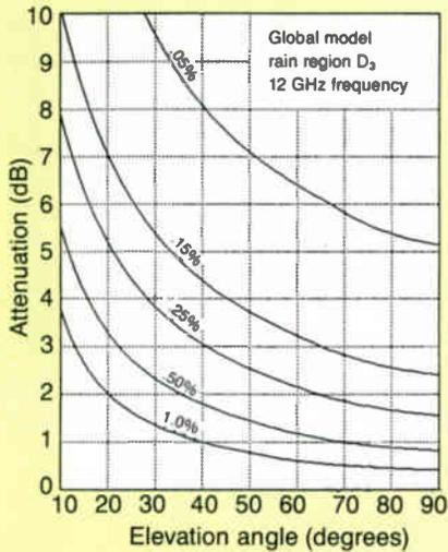
With satellite at 85° W.L., solution of this equation yields an elevation angle of 49°. From Figure 6, rain attenuation is 5.1 dB for 99.95 percent availability.
