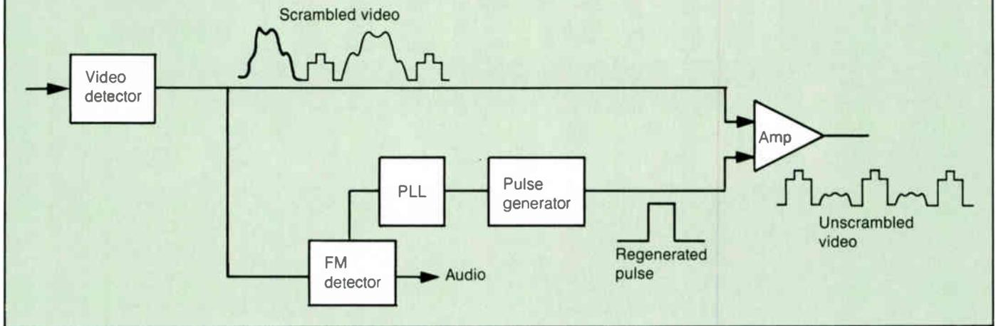
is suppressed below the peak video level. Figure 4 shows a baseband implementation of sine wave scrambling.
