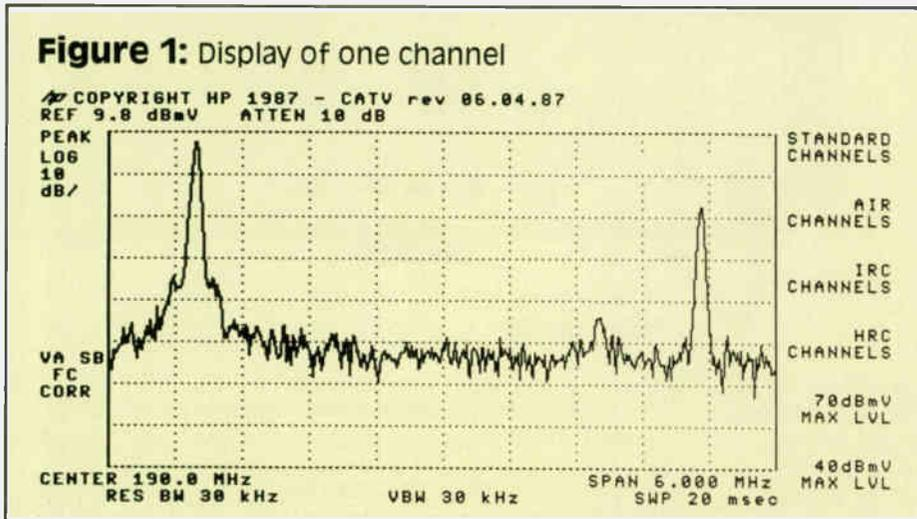
Figure 2: Carrier level measurement
