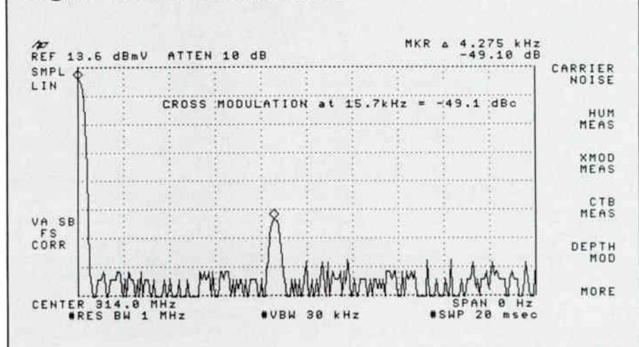
**Figure 6: Composite triple beat measurement**
