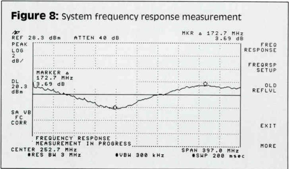
missing bands of channels also can be tested by installing a band-limited noise source at the headend. The analyzer will measure the frequency response of the noise source where the channels are missing in the cable system.
