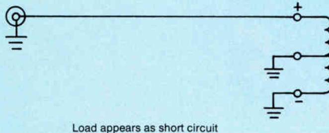
to be employed for unbalanced operation. In these cases, an unbalanced connection may be required to be made to the + terminal while grounding the - terminal, reversing these
