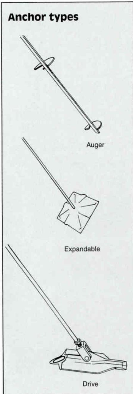
for them, the only equipment to be purchased are drive gads (to drive the anchor into the ground) and the anchor setting device. The cost for this equipment is under \$1,000. The time required for the driving and setting of a drive type anchor is 20 minutes or less in normal soils.
