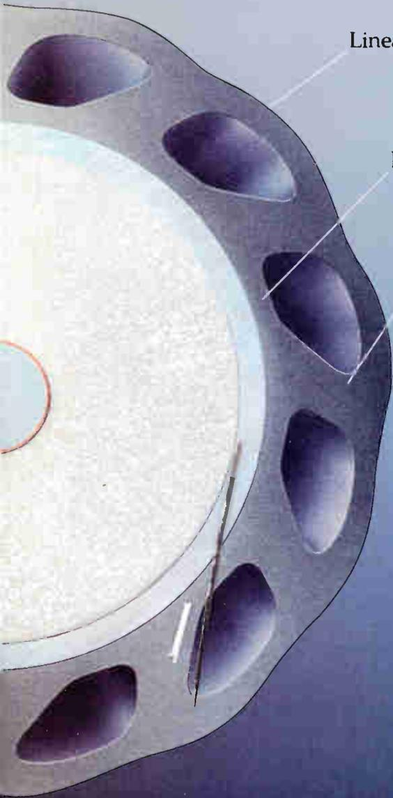
Linear Medium Density Polyethylene Outer Jacket
