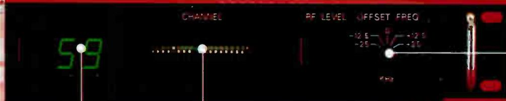
Large green LEDs display accurate channel indication.
