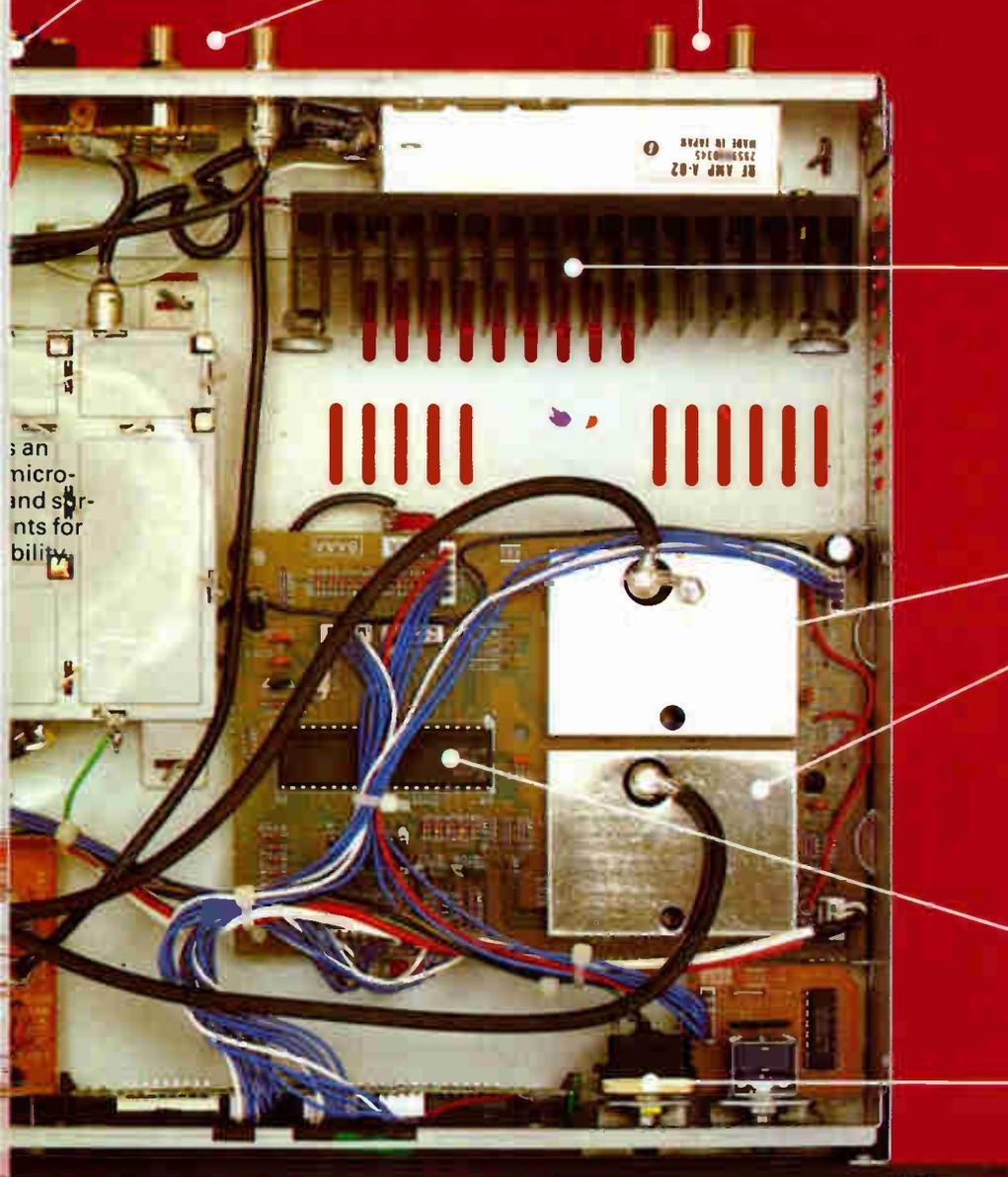
Low noise, hybrid power, push-pull amplifier that is adequately heatsinked and fully shielded.
