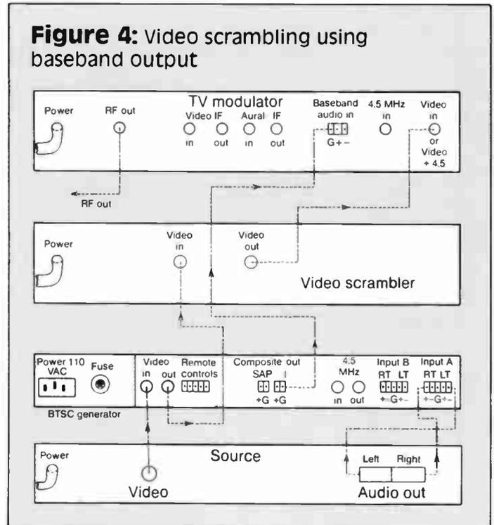
encodes the signal into the BTSC format, which can then be distributed throughout the cable system. A monaural program also may be used as a source. A convenience that then proves to be useful is a built-in stereo synthesizer. With this feature, the ambience is not lost when the program or local ad source is providing mono.
