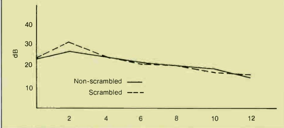
decoder. This was especially significant, considering that this decoder is representative of the type of decoder used by the subscriber. This degradation was most evident when a composite BTSC interface was used; that is, when video and BTSC audio were combined and modulated as a single signal onto a 4.5 MHz carrier. When separate interfaces were used (BTSC on a 4.5 MHz carrier and baseband video as a separate signal), audio/video interaction became imperceptible.
