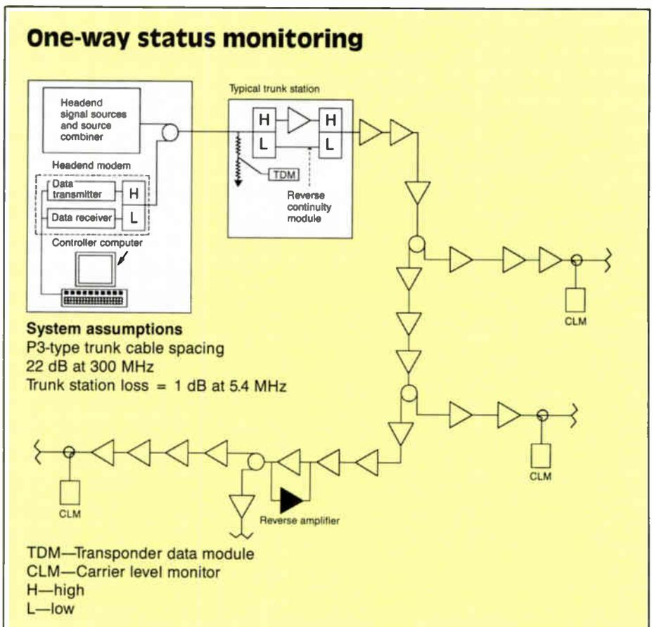
the pilot carrier input levels, which in turn indicate problems in front of the amplifier being monitored. AC power readings indicate potential connector problems or excessive loading. Checking amplifier stations on each side of the power supply will indicate which span is causing the trouble.
