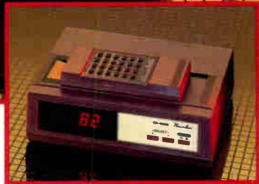
A convenient feature of the CR-6800 is a cradle for the hand held transmitter that provides a storage area for the remote control, and also allows the transmitter to function as an on board keypad to control the convertor.
