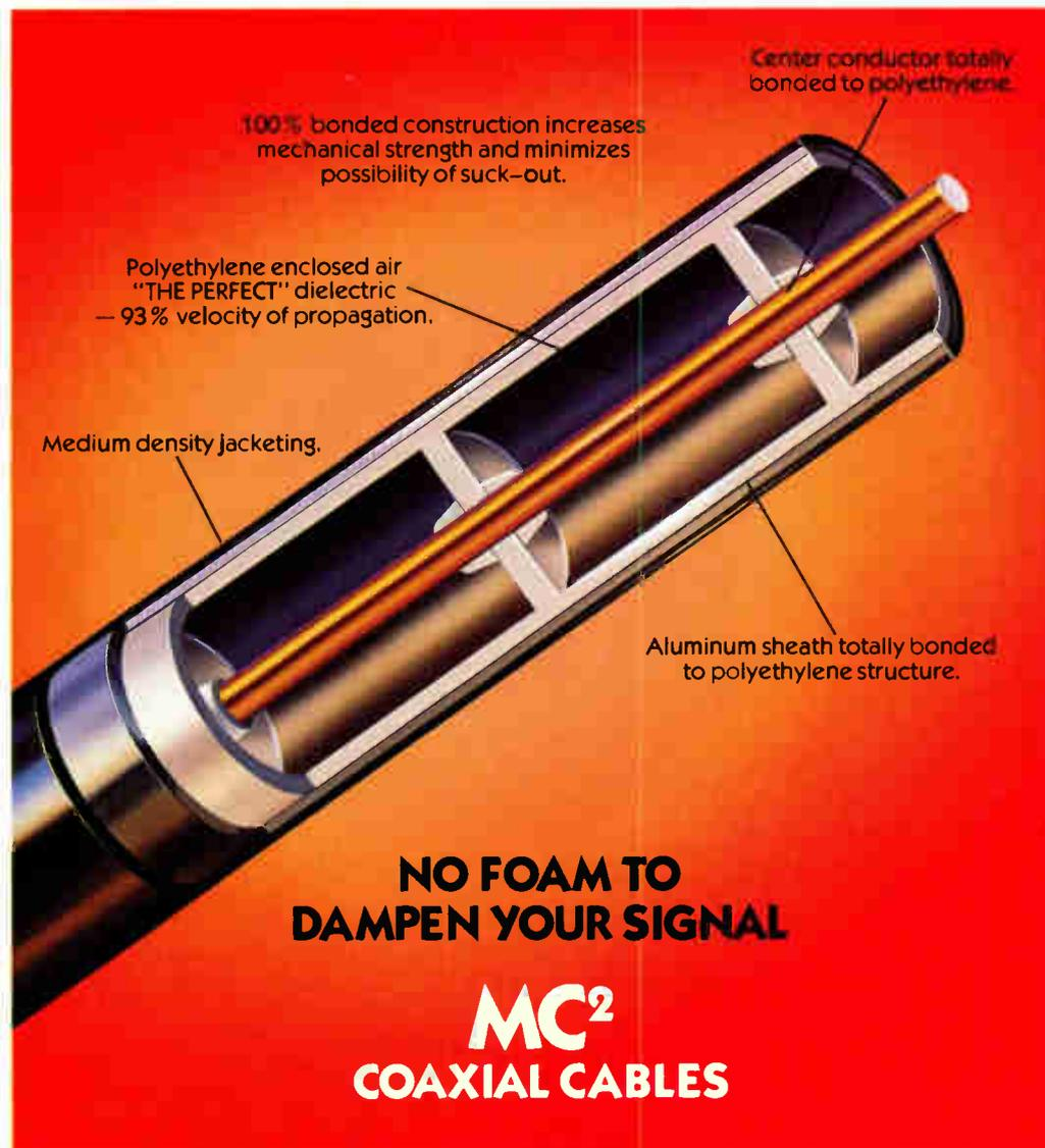
Anyway you slice it, manufacturers of foamed cables have been scrambling to attain the superior attenuation characteristics of MC<sup>2</sup>. The attempt means increasing our familiar MC<sup>2</sup> diameter of .500" to .565" or .625"; and our .750" must become .840" or .860" or .875".
