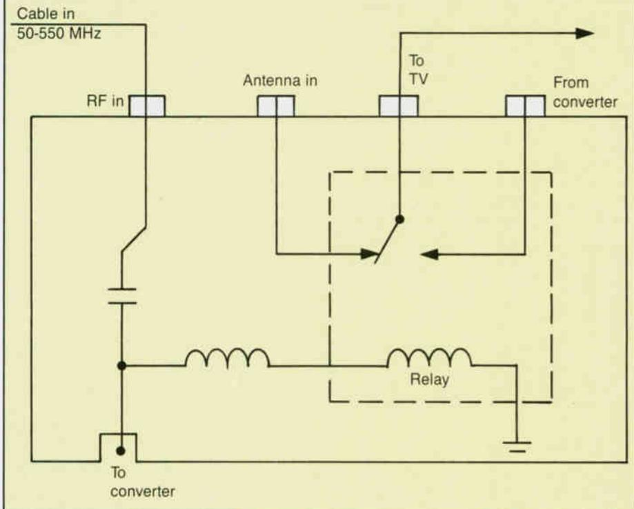
**Figure 7:** Possible output A/B switch option configurations
