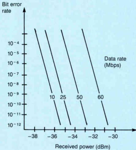
Receiver sensitivity at a particular BER is based on standardized or widely accepted values. However, certain applications may involve either higher or lower BER. Figure 2 also shows how signal power and BER vary for a typical receiver.
