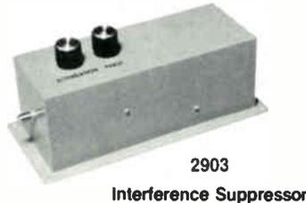
The 2903 co-channel eliminator is a phase cancellation device, used to eliminate or greatly reduce interference caused by co-channel, ghosting, adjacent or FM channels. These types of interference are usually found at or near the same frequency as the desired signal. Phase cancellation is the only practical means of suppressing it.
