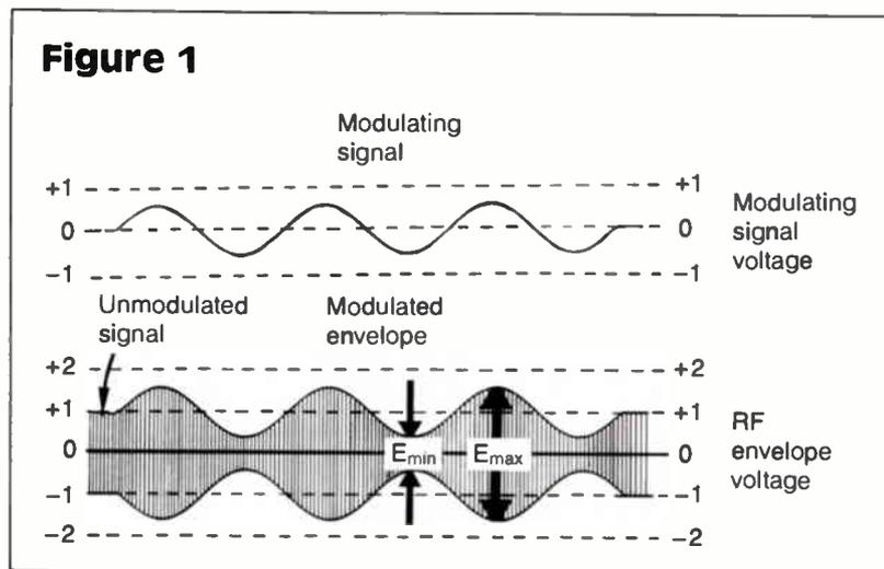
**Problem:** The peak-to-peak voltage of an unmodulated RF carrier's envelope measured on an oscilloscope is 2 volts. If that carrier is amplitude modulated by a 1 volt peak-to-peak signal, what is the percentage of modulation? (Refer to Figure 1.)
