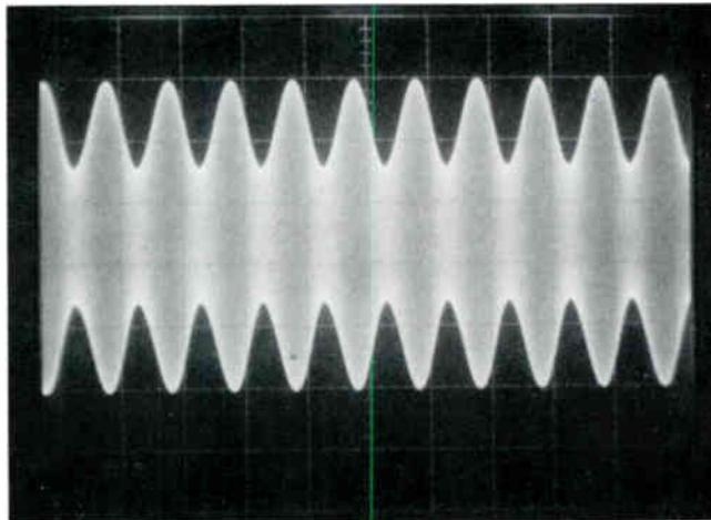
*A 20 MHz carrier amplitude modulated 40 percent by a 20 kHz signal.*
