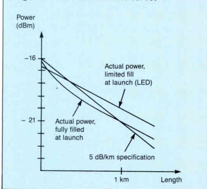
mode distribution exists may cause some power to be coupled into higher order modes, thus causing additional transient loss in the fiber (Figure 1).
