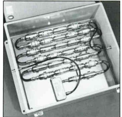
**Typical multitraps assembly. The subscriber-powered amplifier counters cumulative trap loss.**
