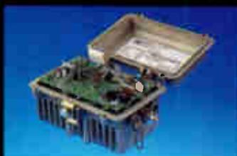
Compact MLM module is enclosed in a rugged housing that withstands the extreme environments of a cable system.
