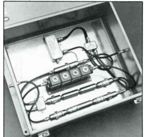
**This multichannel trap assembly uses a special bandpass filter to isolate a desired super-band channel.**
