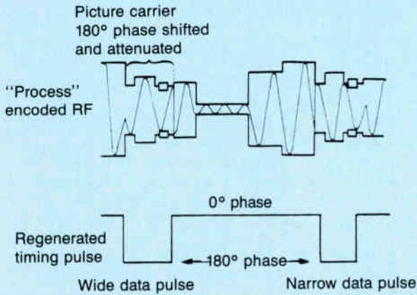
rier at IF (intermediate frequency) in a similar manner to timing pulses for synchronization of RF sync suppression descrambling (Figure 4). Data pulses are transmitted one per line, thus providing data rates approaching 30 kbps. With AM pulses multiplexed on the audio carrier along with timing pulses, critical timing is required to distinguish data pulses from timing pulses.
