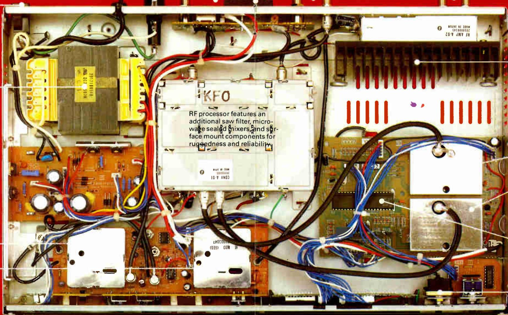
RF processor features an additional saw filter, microwave sealed mixers, and surface mount components for ruggedness and reliability.
