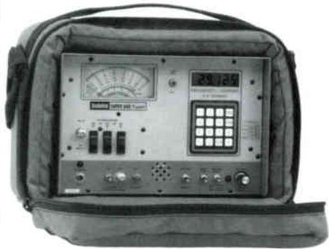
They are the most versatile series of Signal Level Meters and are designed for use at Head-end locations; in the field; in the lab; and on subscriber's premises.
