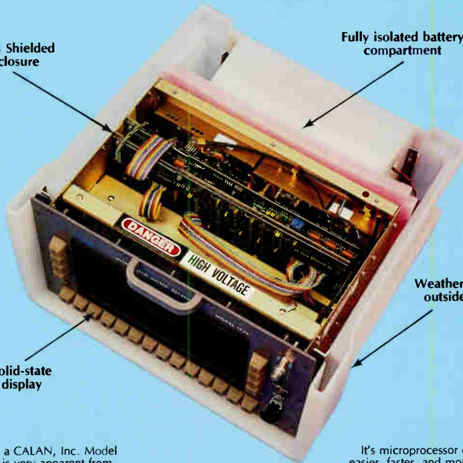
Reliability built into a CALAN, Inc. Model 1776 Sweep Receiver is very apparent from the outside: the totally weather-sealed case; the ruggedized overall construction; the moisture-sealed key covers on the front panel.
