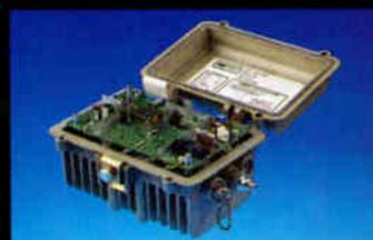
Compact MLM module is enclosed in a rugged housing that withstands the extreme environments of a cable system.
