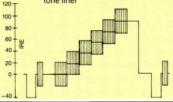
**Figure 3: Digital sampling of video signal**
