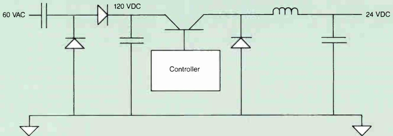
25 to 60 watts under the same operating conditions and substantially more if the wrong primary tap was selected. Under 150 volt surge conditions, dissipation of the 90 percent SMPS unit would be expected to increase only slightly to around 10 watts, while dissipation of SMPS units with AC transformers would increase much more due to core saturation in the transformer. Dissipation of series-regulated linear types can increase to well over 300 watts during the same surge conditions.
