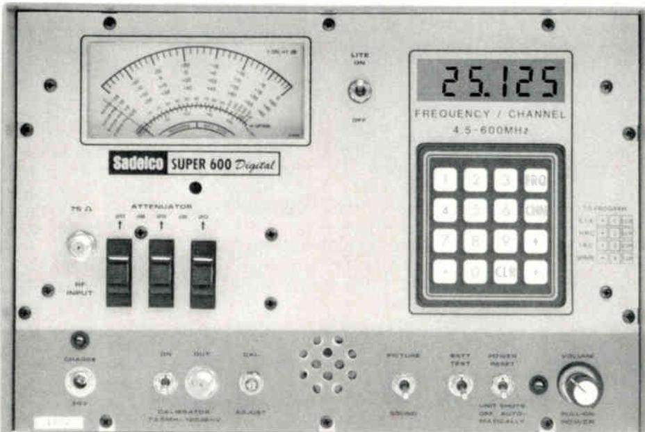
Model Super 600 Digital Signal Level Meter
