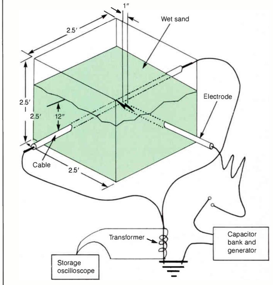
*Siecor armored Mini-Bundle cable* (copolymer-coated ECCS steel armor): No significant damage occurred to the inner sheath and no core damage occurred on this design tested to 115 kA. Only the outer jacket and armor was penetrated at current levels as high as 150 kA. At higher levels, to 229 kA, only minor damage occurred to the inner jacket and again no core damage occurred.
