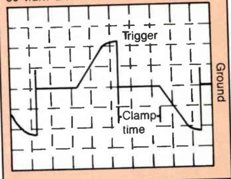
could get rid of. The voltage across the SCRs when conducting is only 0.3 volts. It does not even show as such in Figure 7 where you can see an overvoltage of about 220 V instantaneous taken to within 0.35 volts of sheath ground in a matter of nanoseconds.
