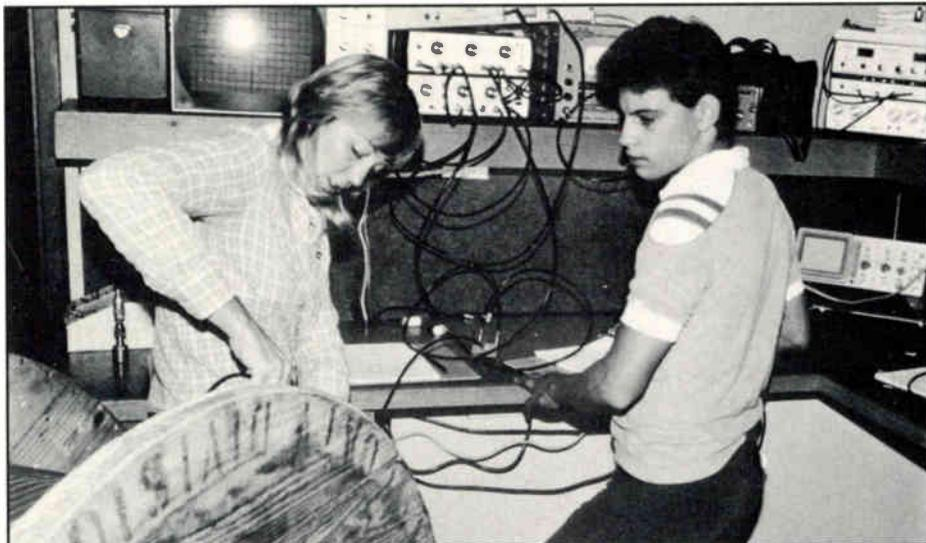
At the ATC National Training Center students use sweep test equipment to perform a return loss test of coaxial cable.
