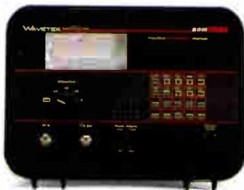
CAL feature permits instant field calibration for temperature variations and test probe, and it even shows when an error in calibration has occurred.
