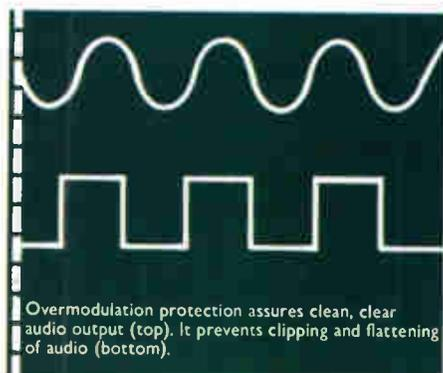
Overmodulation protection assures clean, clear audio output (top). It prevents clipping and flattening of audio (bottom).
