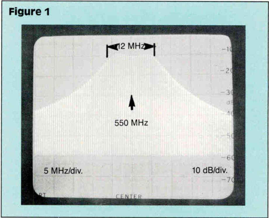
loss of the multistage UHF filter network will in turn reduce the carrier-to-noise ratio of the signal by 2 to 3 dB, a sometimes unacceptable reduction in performance.
