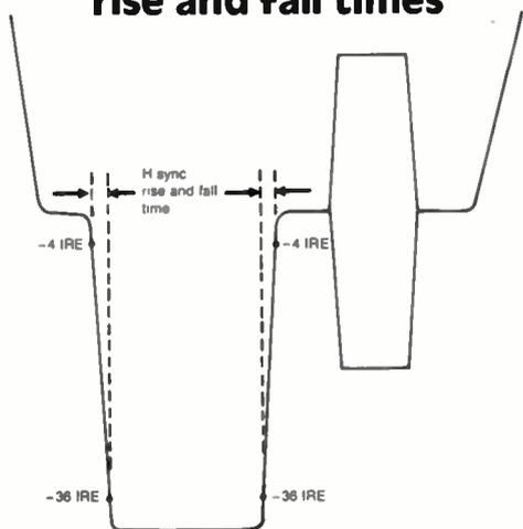
The rise and fall times of horizontal sync—measured between the 10 and 90 percent points on the pulse leading and trailing edges—are not to exceed 0.250 microsecond.
