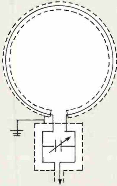
of the leak instead of the electric field. The magnetic field has a more pronounced attenuation effect with distance and does not seem to exhibit the same extreme standing wave effects that electric fields demonstrate.
