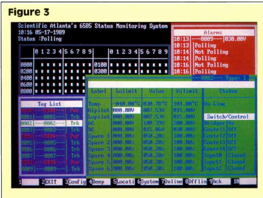
mal downtime. One of the tools to achieve this goal is the selection of reliable distribution equipment. An additional tool is the use of status monitoring (SM) in the distribution plant for early detection of problems, trend analysis, analog measurements, as well as ingress control. An emphasis on the human interface is essential as the system is used and operated by non-technical personnel (i.e., dispatchers).
