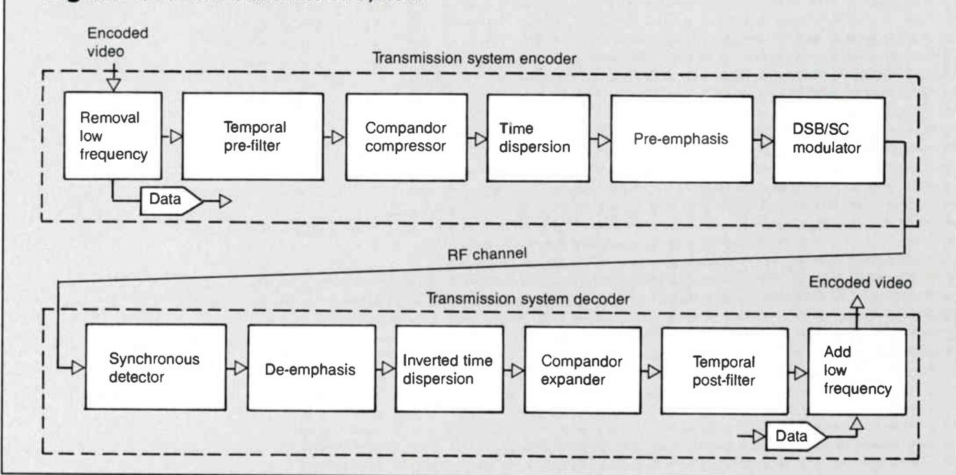
**Figure 2: SC-HDTV receiver multimedia operation**
