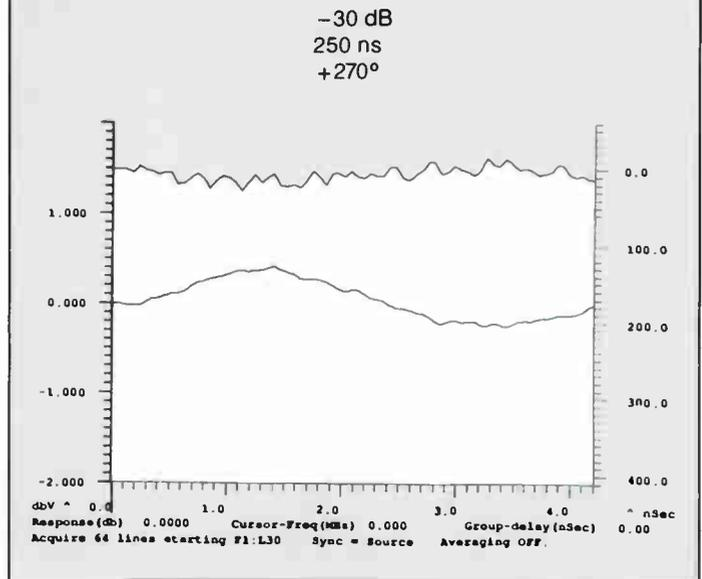
passive devices. The drop termination is generally considered a relatively poor match of only a few dB, and the potential exists, especially in cases with splitters feeding extra outlets, for reflections in the 100 ns range in excess of the threshold of perceptibility for either of the impairment functions.
