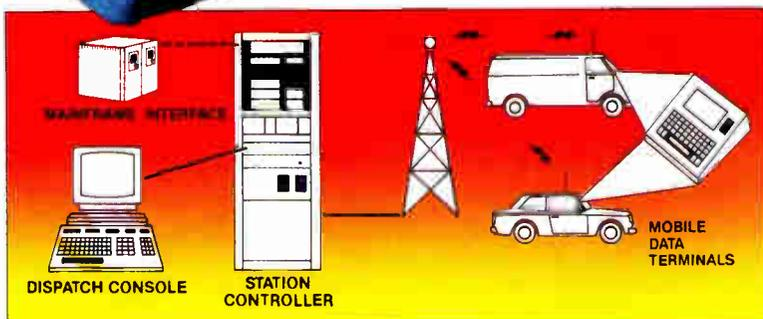
The C•ARDS System - the dispatch console includes a microcomputer which houses specially-designed software, terminals, keyboards and printers. The station controller contains equipment which interfaces the microcomputer to your billing system and existing radio base station. Mobile data terminals in each vehicle enable operators to communicate with the dispatcher, send information and access data stored in the microcomputer or a host computer.
