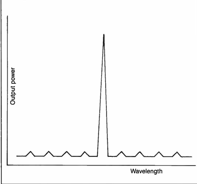
quantum wells and usually a single mode of operation is achieved, with a line width narrower than that of current DFB lasers. Another benefit of quantum well structure is a very low threshold current, enabling operation of the laser with less external electronics.
