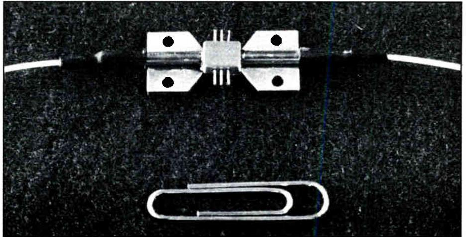
**The diode laser amplifier is the only optical amplifier commercially available.**
