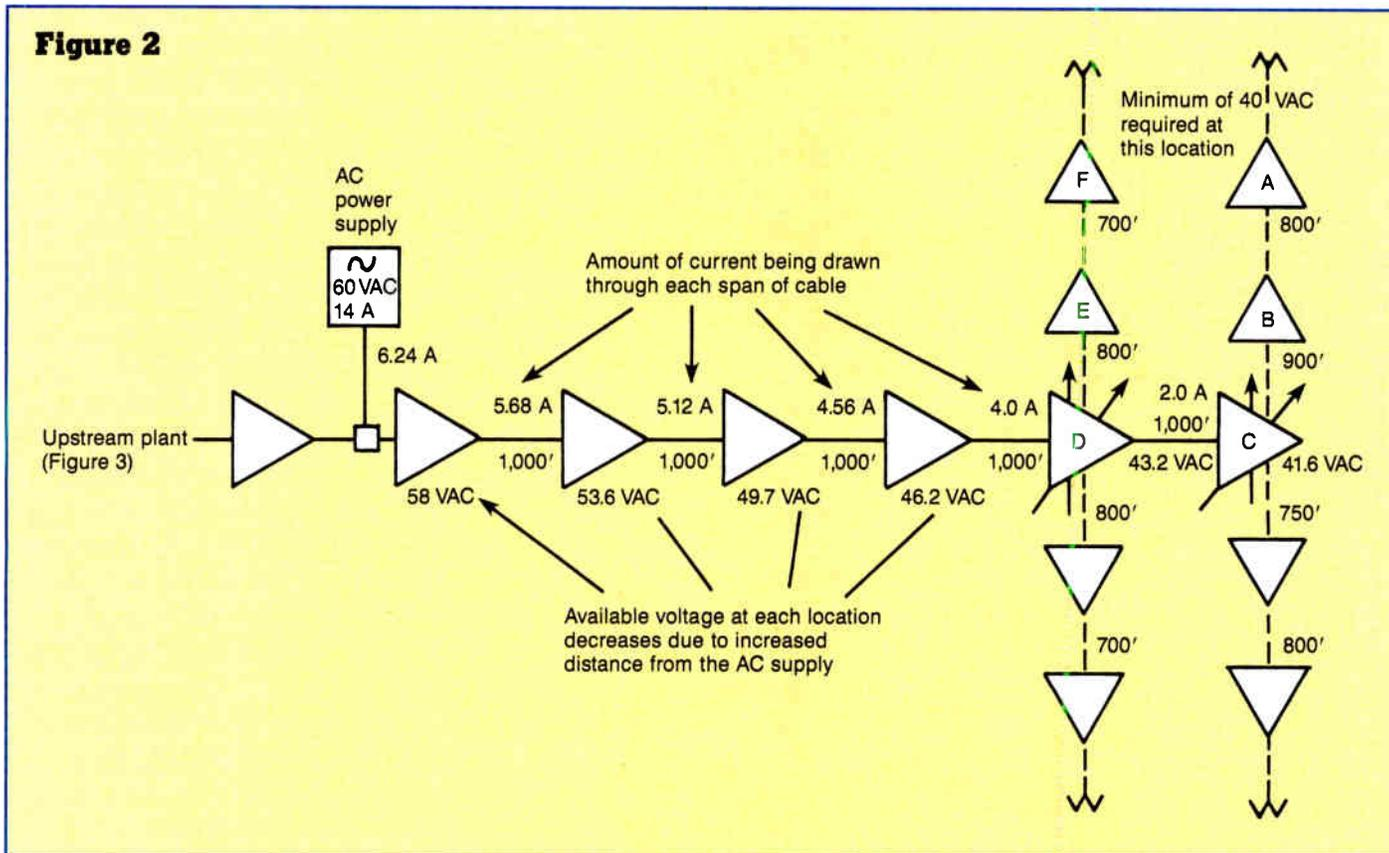
for any eventual additions to the system and the AC power supply will not have to be relocated. Also, it is not wise to allow more than about 6 A of current to flow through any amplifier. Of course, this applies mainly to the amplifiers closest to the AC supply.
