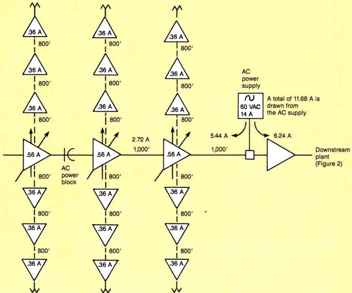
plying  $1.5 \Omega$  by  $0.72 \text{ A}$  we calculate a drop of  $1.1 \text{ V}$  (rounded off). The required output voltage at the bridge/trunk is  $41.6 \text{ VAC}$ . Keep in mind, we are working upstream toward the AC power supply location so that the voltage levels at each amplifier will increase.
