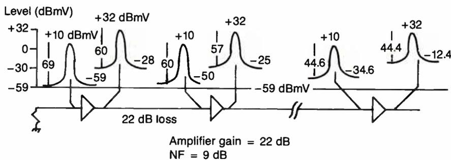
**Figure 2: Correction for determining plant noise**
