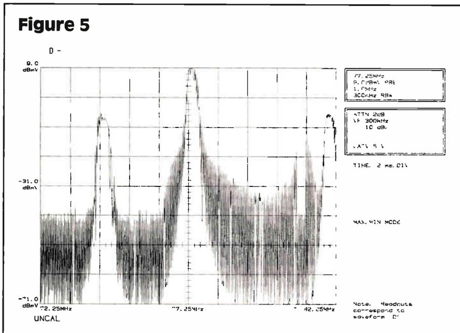
by 10 dB, an increase of 10 dB in C/N capability is obtained. This capability exists in some analyzers, but may cause spurious signals to appear on the screen. Since this measurement is one of carriers and noise, the spurious signals (if present) can be ignored. A typical analyzer has a noise figure of 30 dB that calculates to a maximum C/N capability on a +10 dBmV signal in a customer's home of 36 dB without using external preamplifiers.
