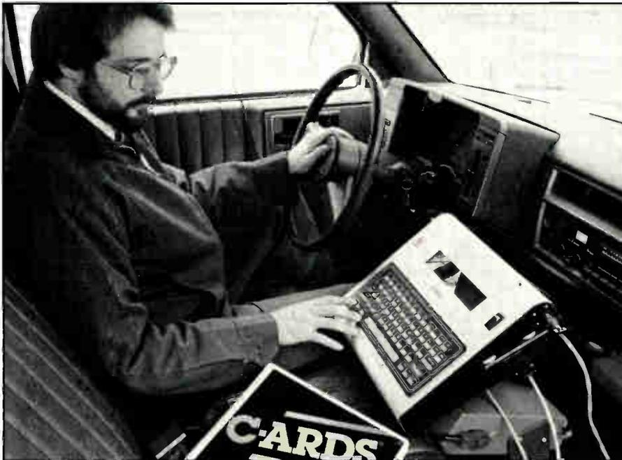
The service tech completes a work order and sends a message via the C-ARDS terminal to dispatch.
