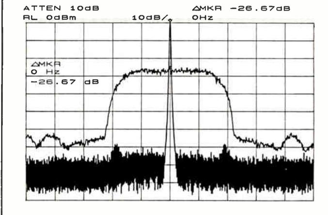
The mean power level equation is solved by exponentiating the value of the main lobe power level, multiplying it by the factor (Fs/BWn), taking 10 times the log of the product and adding the 2.5 dB correction factor. (See lines 1130, 1140, 1150 and 1160.)
