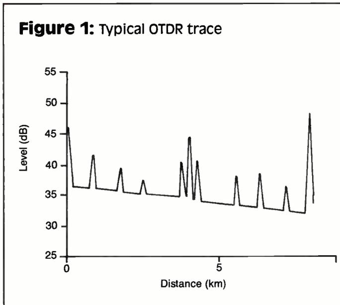
Figure 1: Typical OTDR trace
