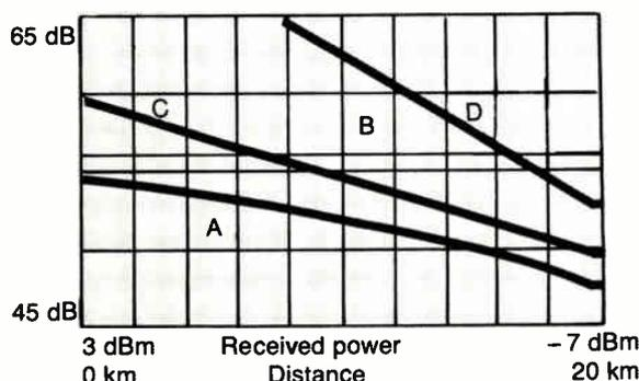
A—link CNR. B through D are CNR due to: B—laser intrinsic noise, RIN = -153 dB/Hz, C—photodiode quantum noise, responsivity = 0.85 A/W, D—amplifier noise, R<sub>1</sub> = 1,000 ohms, F = 3 dB. Laser output is 2 mW and modulation index is 0.04/channel. Fiber loss budget is assumed to be 0.5 dB/km.
