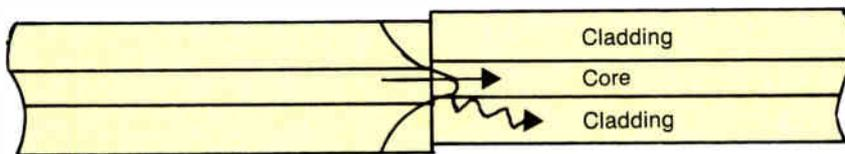
**Figure 2: Mechanical splice**
