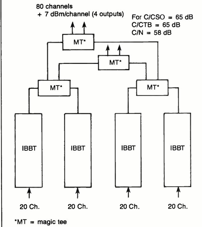
tively few receive sites so four outputs at +7 dBm per channel would suffice. The IBBT is operated with 32-channel output level approximately 2.5 dB above that implied by the table, so that C/CTB would be 60 dB, C/CSO would be 62.5 dB and transmitter C/N would be 64 dB. The result is a 64-channel transmitter with four output ports; a more cost-effective solution than adding four complete racks of MTX-132 equipment.
