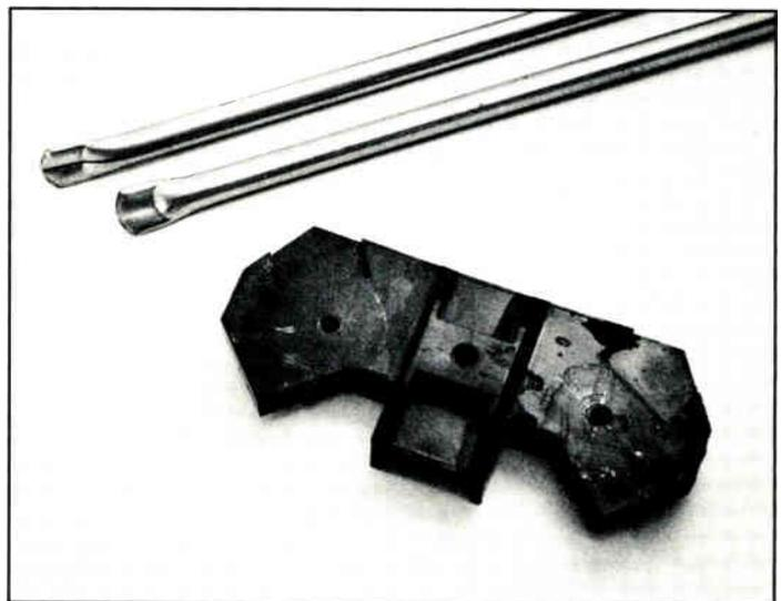
**Photo 1:** Drill out the rivets that hold one of the plastic brackets and a pair of elements to the TV antenna's boom. Use the longest elements, each of which should be about 4 feet long. The plastic bracket will be the dipole's center support, and the two TV antenna elements will be fabricated into the dipole's two elements.
