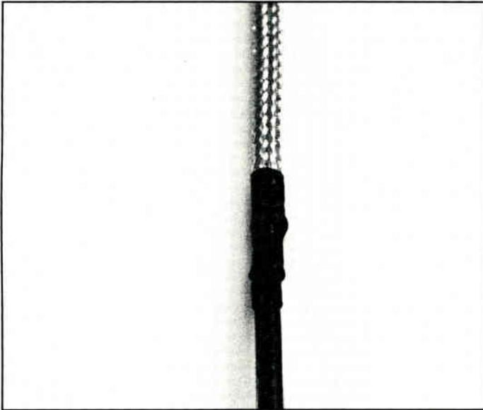
**Photo 9:** Install a small piece of heatshrink tubing over the solder connection and shrink it with a blow dryer.
